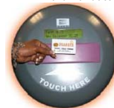
Figure 2: Toll Lane Smart Card Validator
