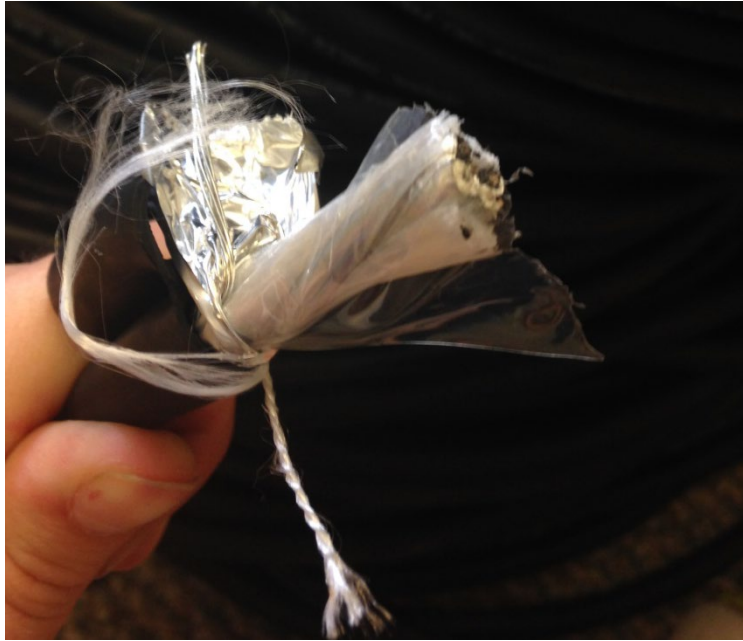
Figure 3.24 Double shielded wire
