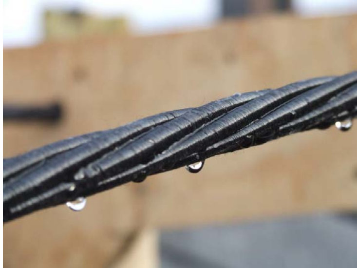
Figure 1. Water Drops on a Corrosion-Free Carbon Fiber Reinforced Polymer Strand
