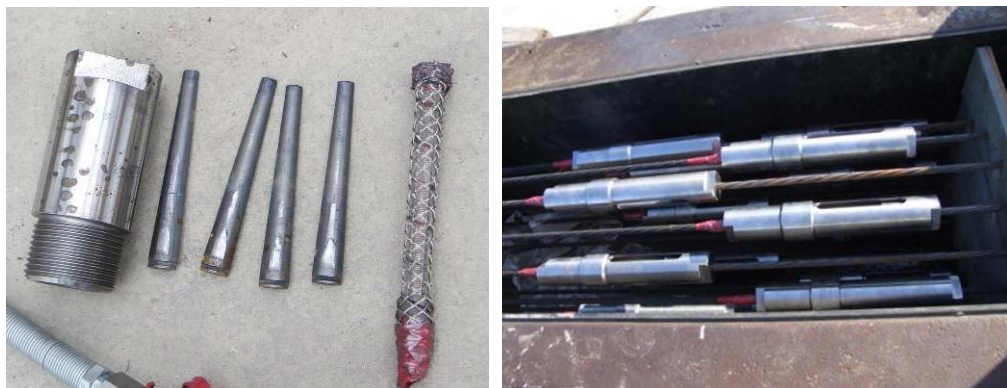
Figure 3. Elements of End Preparation: left, disassembled wedge, chuck, and braided grip; right, couplers in a pile
