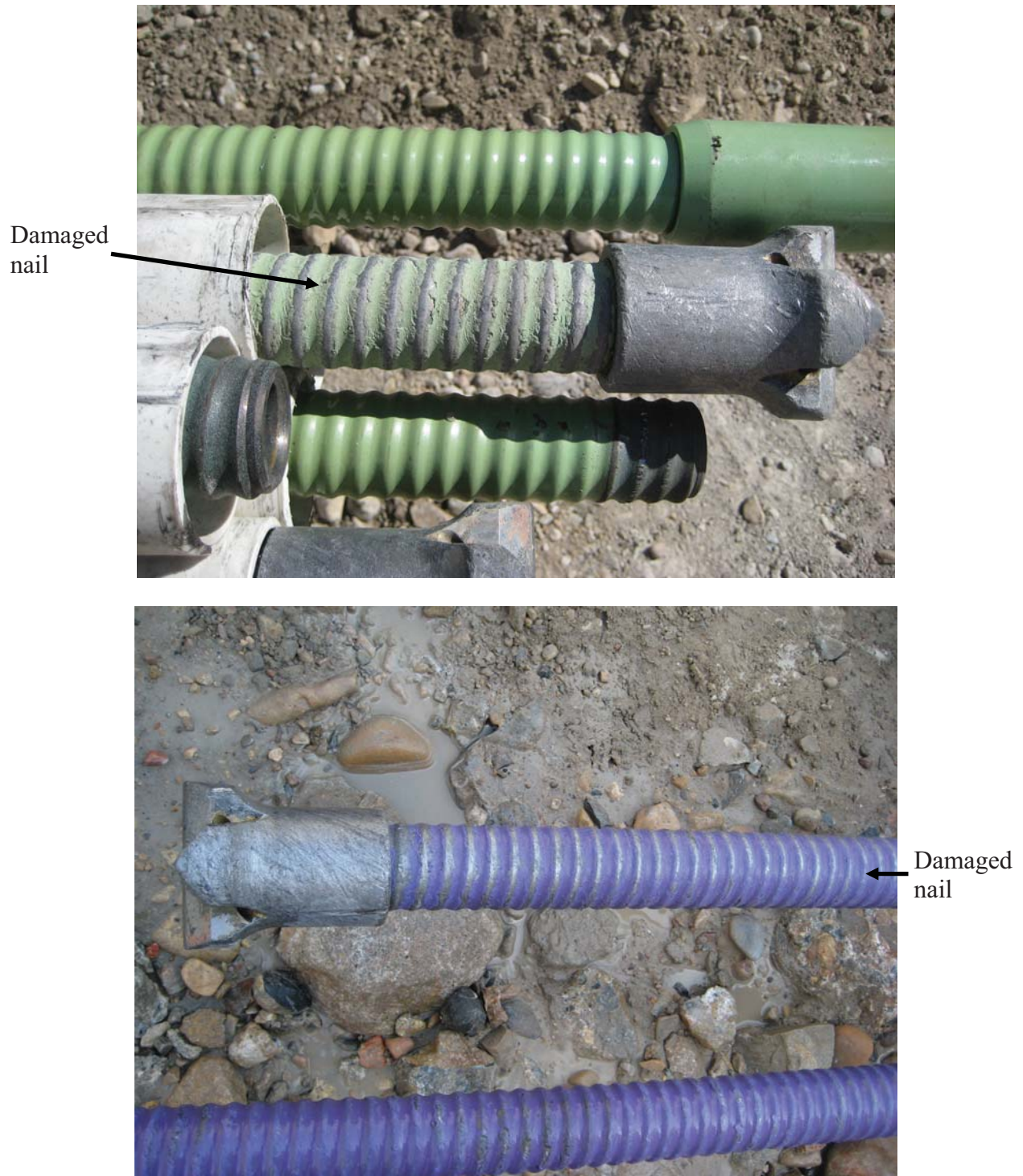
Figure 1. Photo. Damage to epoxy coatings (Courtesy: Schnabel Engineering/ADSC).
