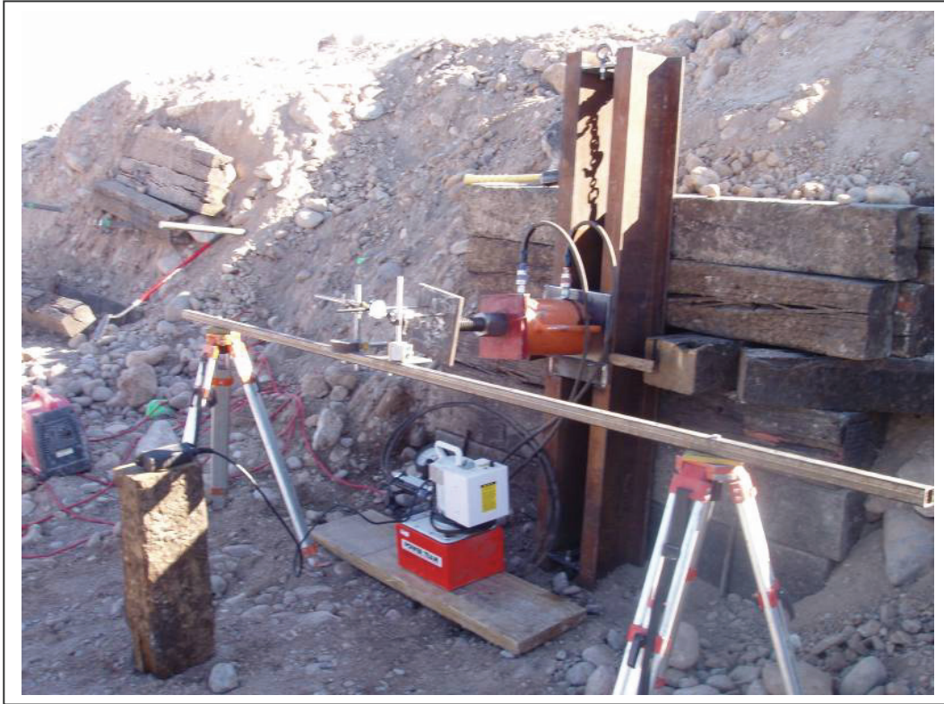
Figure 12. Photograph. Load test setup at Sunset Mesa Site.
