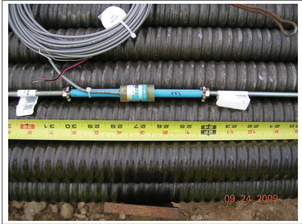
Figure 9. Photograph. Geokon Model 4200-AX strain gauge with threadbar attachment and notched dumbbells.
