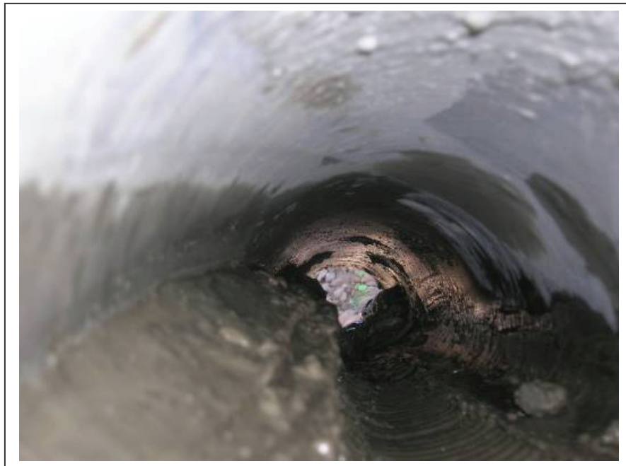
Figure 5. Photograph. Grout remaining in the casing after flushing at the Sunset Mesa Site.
