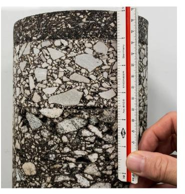
Figure 1. Picture of a thin asphalt overlay.
