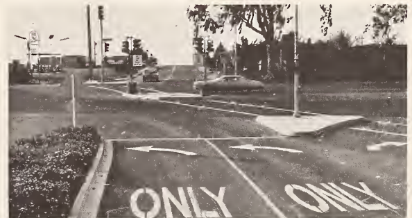
Figure 43. Forced turn channelization — Richmond, CA.
