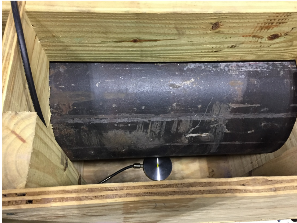
Figure 58. The sand compartment before filling with sand and the pressure sensor is bonded at the bottom with double-sided tape.
