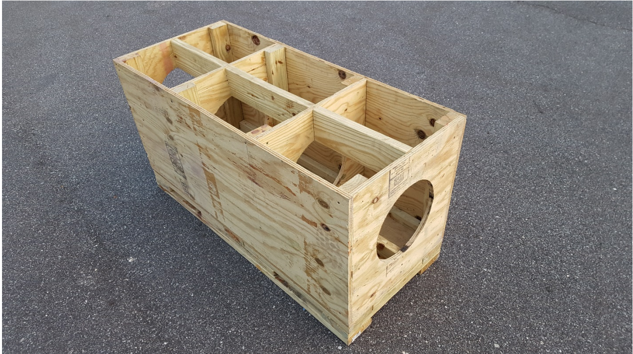
Figure 56. Buried Pipe Test Box for the soil test of the 12-in steel pipe.
