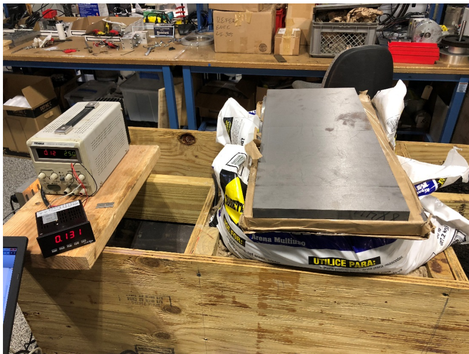
Figure 60. The sand compartment with applied deadweight on the top.
