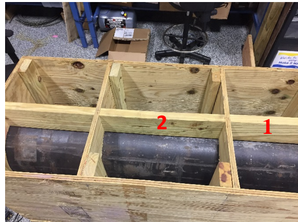
Figure 57. 12-in pipe in the empty buried pipe test box.
