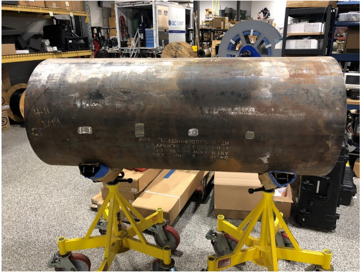
Figure 34. A photo shows the 24-inch ERW pipe with the local wall thinning defects facing to the front.
