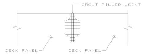
Figure 3 Detail sketch of a female-to-female type shear key transverse joint.
