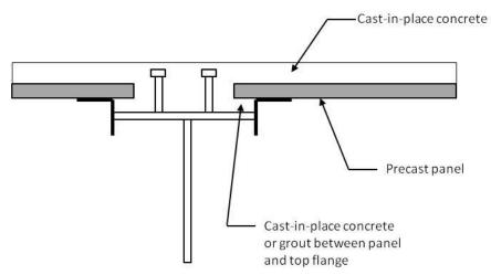
Figure 4 Partial-depth precast concrete deck panel.
