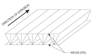
Figure 19 Example of an aluminum deck panel created by welding rib extrusions together at the top and bottom flanges of the extrusion (24).
