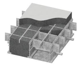
Figure 11 Filled Steel Grid Deck (courtesy of BGFMA (11)).
