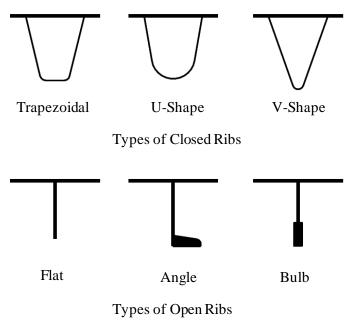
Figure 15 Common Rib Types for Orthotropic Steel Decks.
