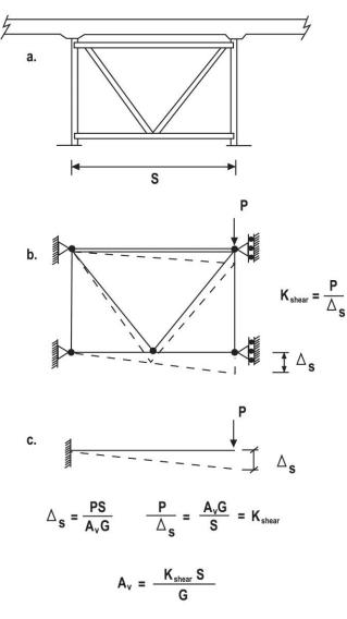
a. K-frame, b. Plane-frame or Plane-truss model,
