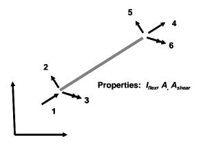
Figure 16 Plane Frame Element.
