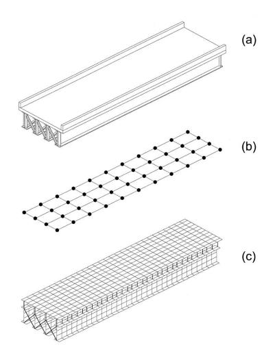
Figure 15 Rigorous analysis method models. (a) Actual bridge, (b) 2-D, or "Grid" analysis model, (c) 3-D analysis model.
