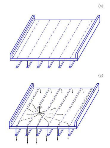
Figure 1 Illustration of live load distribution. (a) Basic girder bridge, (b) Distribution of a concentrated load such as a wheel load through the deck to various girders and then to the girder supports (after Ref. 15).
