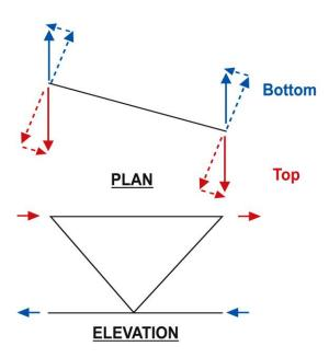
Figure 10 Detail of skewed cross frame deflections during girder rotation.
