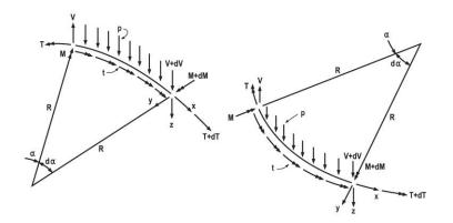
Figure 14 Basic free-body diagrams of the M/R method (6).
