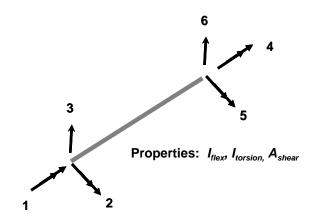
**Figure 17 Plane Grid Element**
