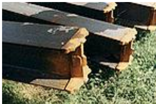
Figure 5 Example of pile tips.
