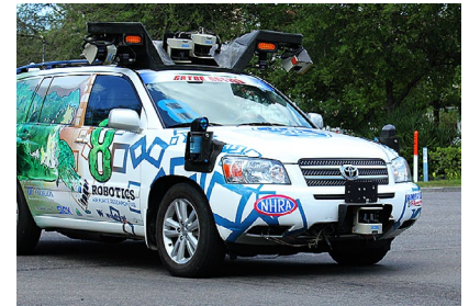
This experimental vehicle is part of a FDOT initiative to test CAV technologies. Components, such as sensors and communication devices, normally built in a vehicle, are exposed for testing purposes.
