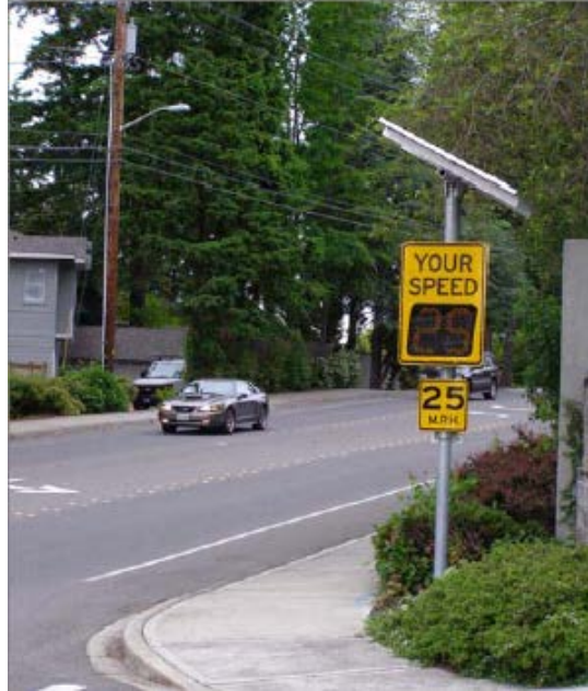
Figure 4. Photo. DSFS system in Bellevue, Washington. (24)
