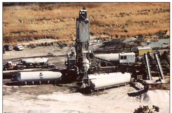
Figure 8-1. Portable concrete plant (ACPA)
