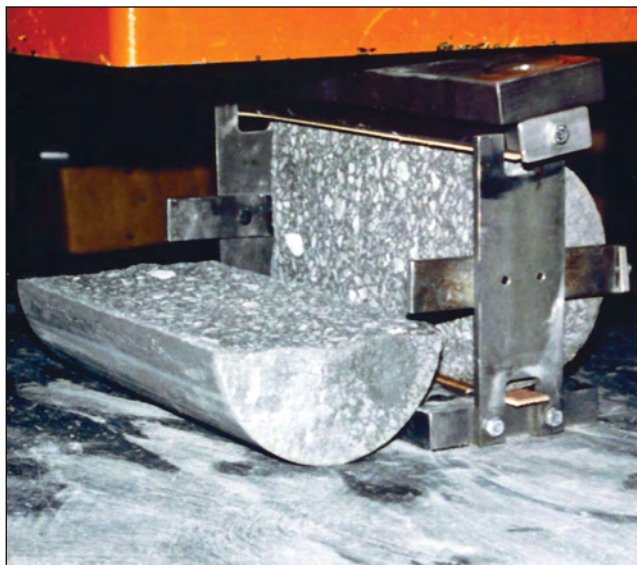
Figure 5-7. Splitting tensile strength (PCA)
