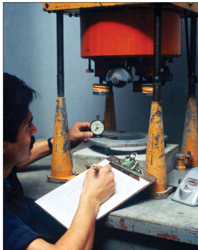
Figure 5-20. Test apparatus for measuring abrasion resistance of concrete to ASTM C 779 (PCA)
