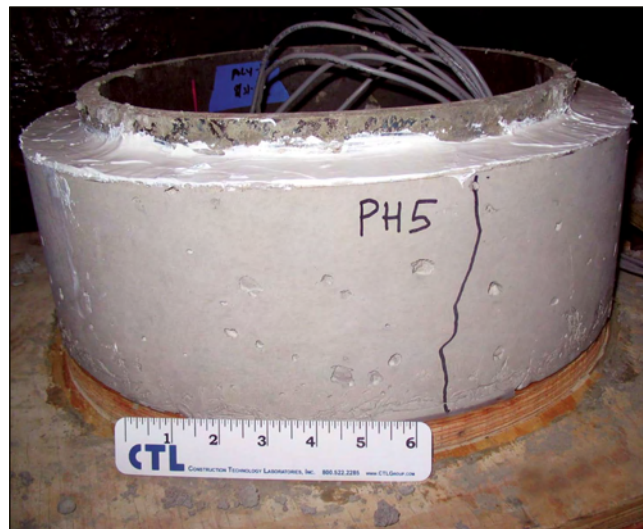
Figure 5-29. A ring shrinkage specimen marked where a crack has occurred (CTLGroup)
