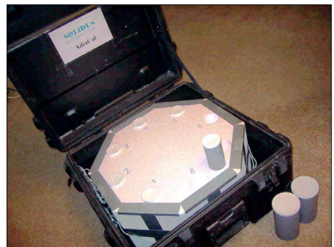
Figure 5-12. A typical field semi-adiabatic temperature monitoring system for mortar (W.R. Grace & Company)
