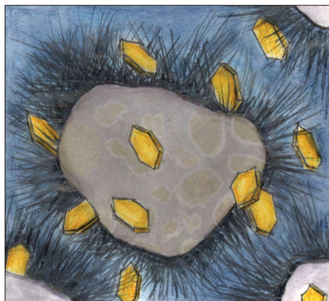
Figure 4-10. Hydration products grow during cooling.
