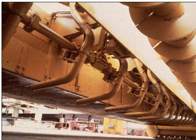
Figure 8-9. An array of vibrators under a slipform paver (ACPA)
