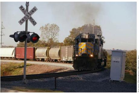
Figure 4. Photo. Highway-railway grade crossing and flashing lights.
