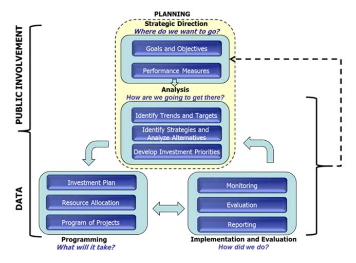
Figure 1. Performance-based transportation planning process.
