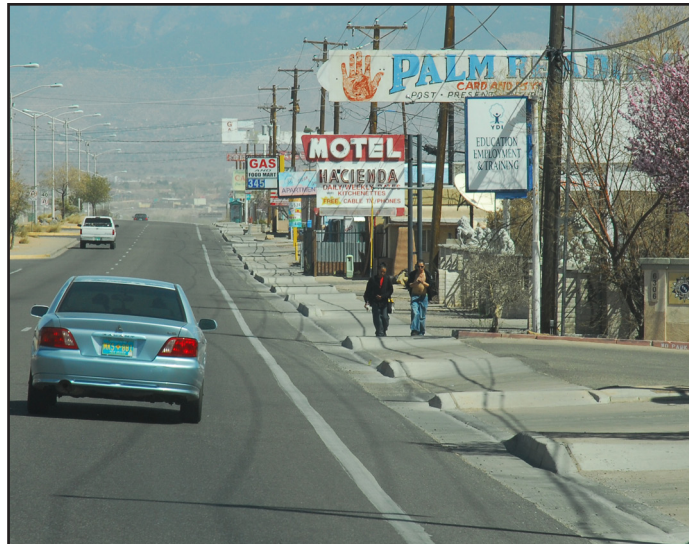
Exhibit 14: A corridor with closely spaced driveways creates a challenging environment for pedestrians and bicyclists. Pedestrians with mobility restrictions may be particularly affected by driveways through sidewalks. These locations require careful design and construction to ensure they meet requirements under the American with Disabilities Act (ADA). (Source: VHB)
