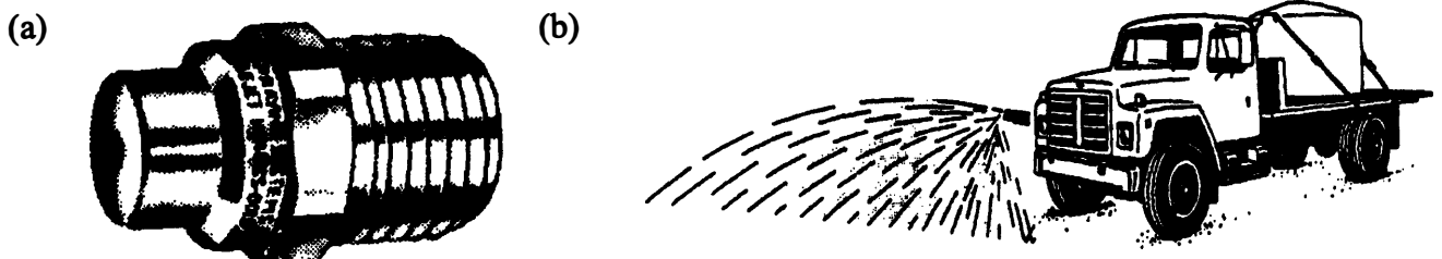
Figure 10.19 The solid-stream nozzle (a) is used for making boomless broadcast herbicide applications (b).
