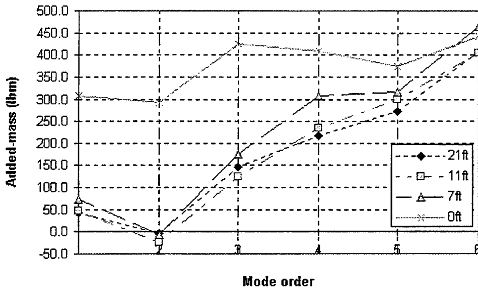
Figure 133. Added mass as a function of water heads
