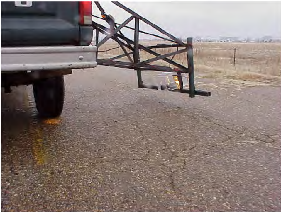
This high speed video camera is observing sand particle movement.
