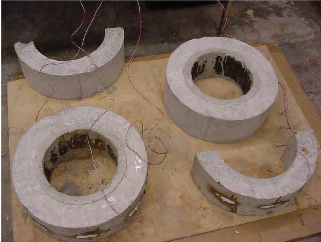
The ASTM 14-day Ring Test examines the cracking potential of concrete mixes.
