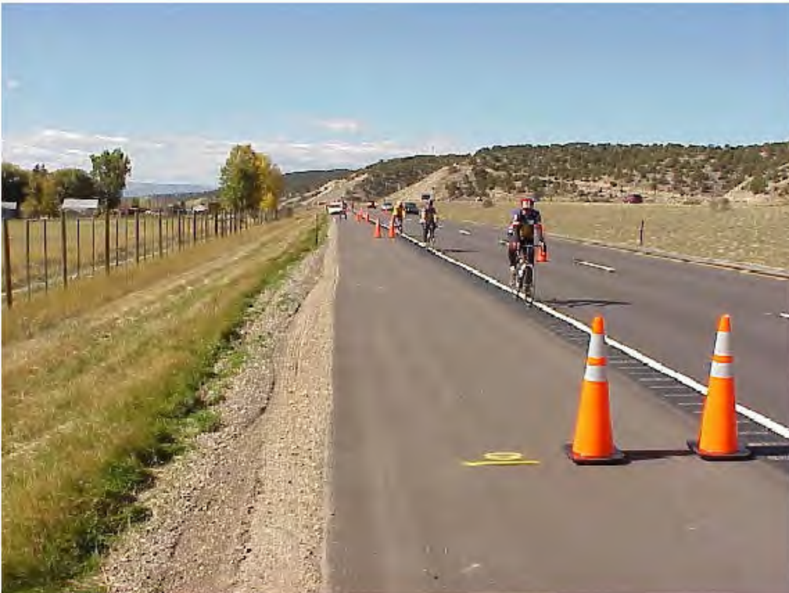
Bicyclists test rumble strips placed along side the edge of the road.
