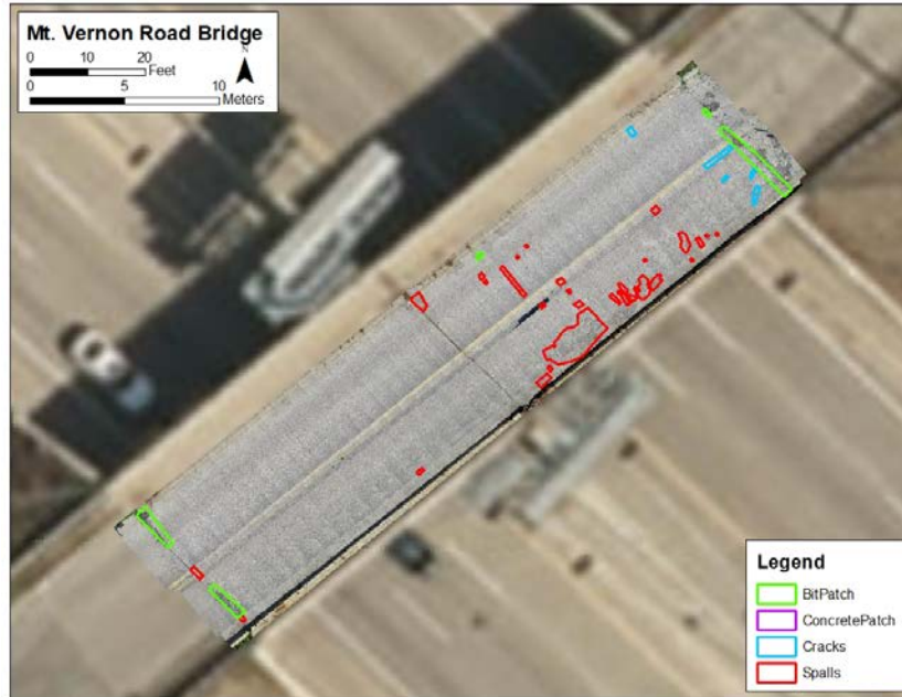
Figure 4. Identified distresses on the Mt. Vernon Road bridge.
