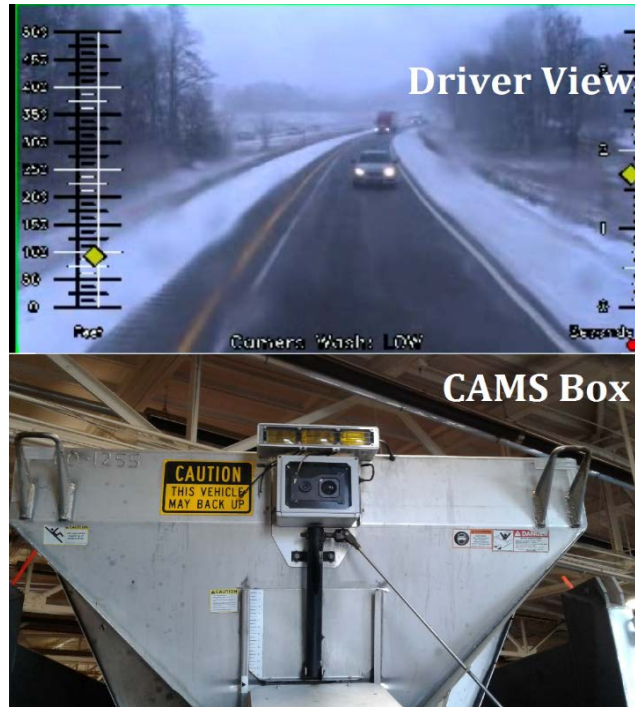
Figure 3-1 Collision Avoidance and Mitigation System
