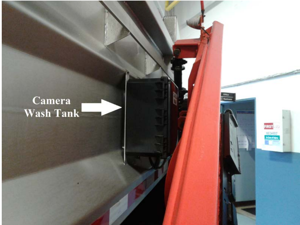
Figure 7-1 Camera Wash Tank
