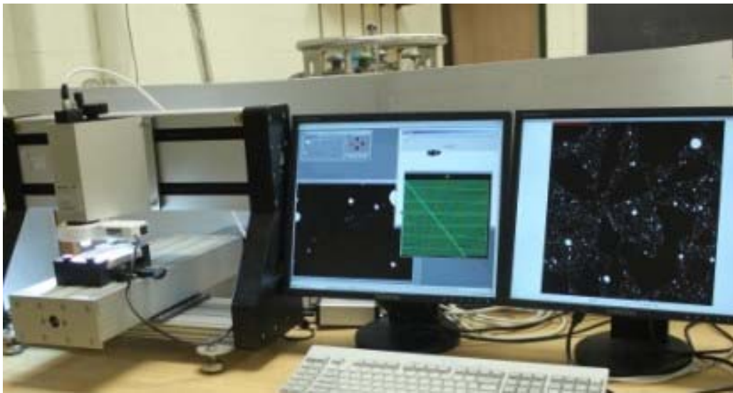
Figure 4-5 Photograph of the linear traverse method point count instrument
