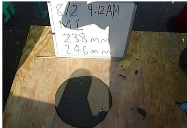
(f) Flow test on UHPC
