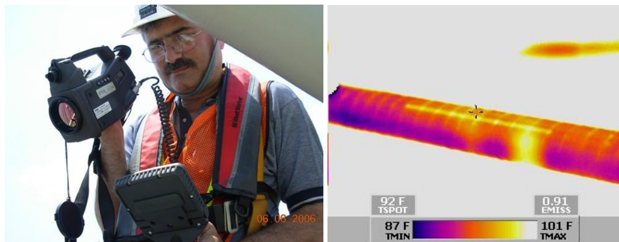
Figure 21: Figure 23: Infrared Thermal Imaging; Use of IRT camera (left) and a thermal image (right) [61]
