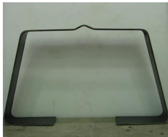
Figure 2. Typical Cross Section for Folded Plate Girder.
