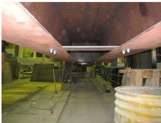
Figure 5. Bottom view of 46 ft. Long folded plate girder.
