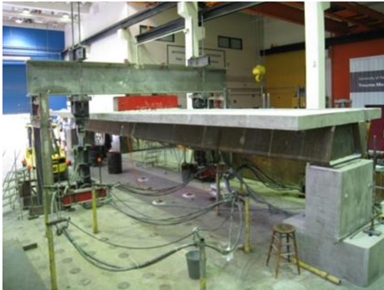
Figure 8. Composite Test Setup.
