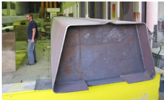
Figure 3. 46 ft. Long Folded Plate Girder.
