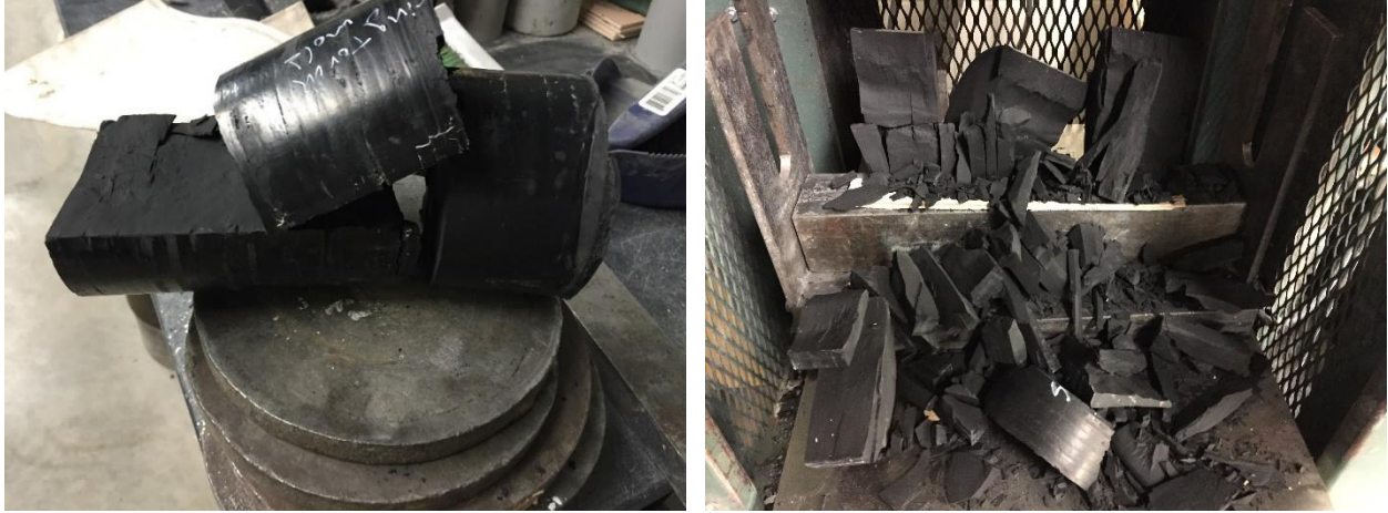
Figure 11. Failure planes for split tensile test specimens made via spring-form mold (shown in the testing apparatus on the right)
