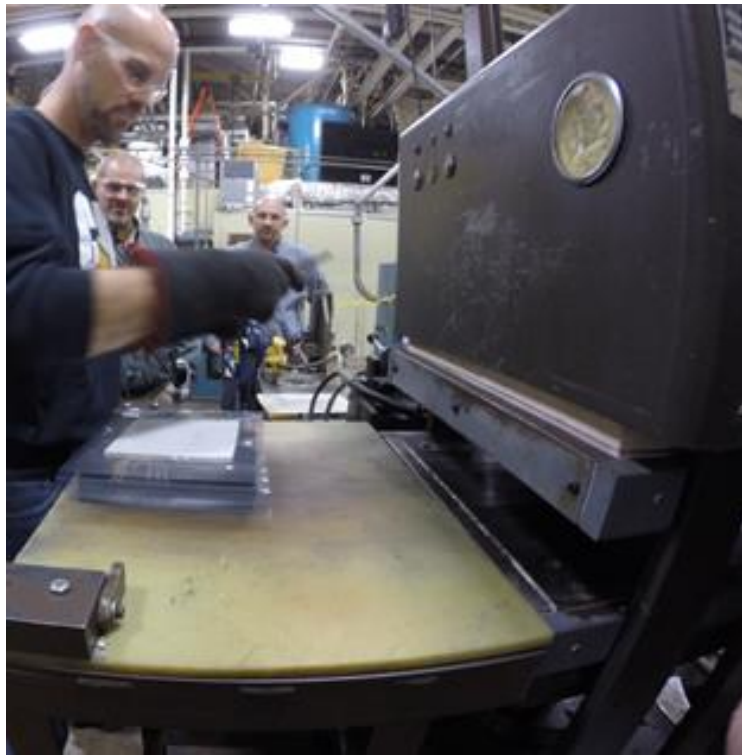
Figure 7. Mold and heated press process
