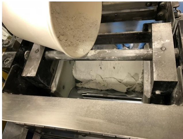
Figure 5. Addition of fillers during mixing process
