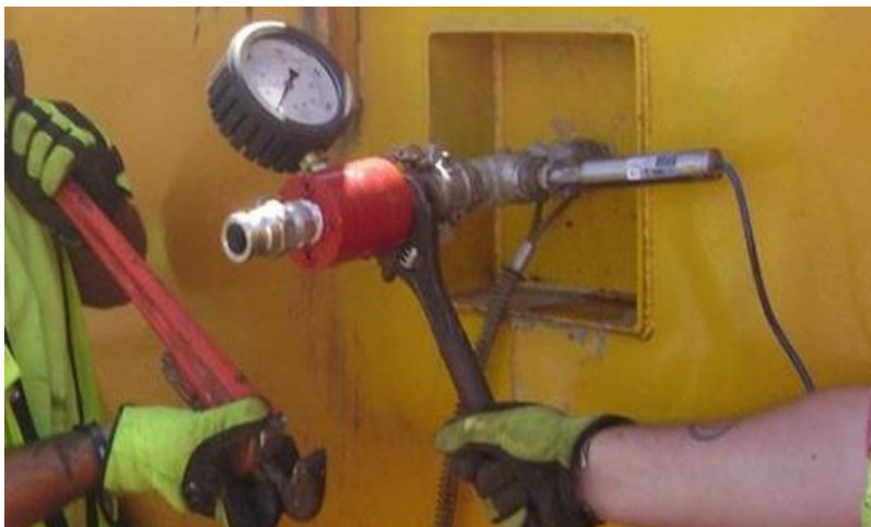
Figure 6.1: Photograph of a Bourdon-type pressure gauge and a pressure transducer (courtesy of Applied Foundation Testing).
