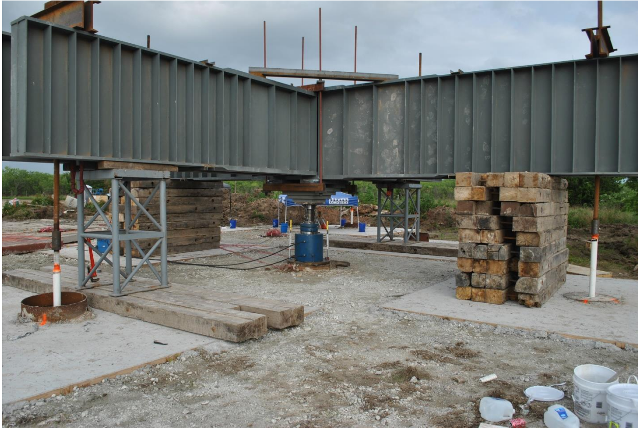
Figure 10.7: Load test setup for top-down loading.
