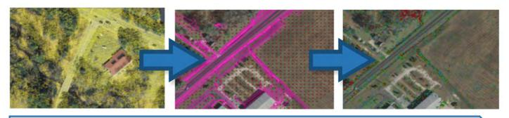
Data Source: 3D Cloud Point Aerial Imagery **Process:** Add Breaklines and Mass Points Extract Topographic Features Final Product: QL2 Bare Earth Point Cloud DTM (Breaklines/Mass Points) CADD Topographic Drawing
