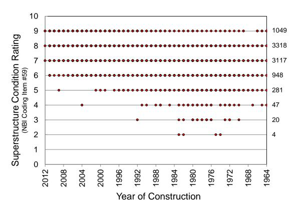
Figure 11. Graph. Superstructure condition ratings of uncoated weathering steel bridges by year built.
