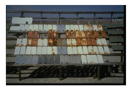
Figure 3. Photo. Testing of various generically similar paint systems shows wide variations in performance.
