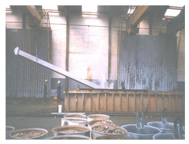
Figure 7. Photo. Hot dip galvanizing kettle with long beam being dipped at one end.
