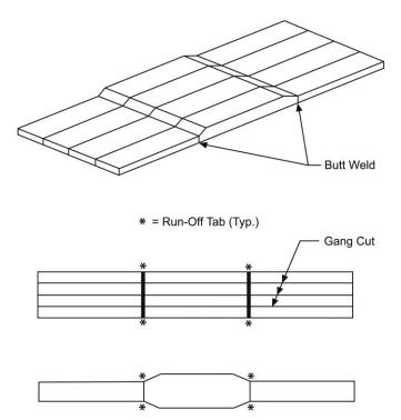
Figure 6 Sketches showing the slabbing and stripping process
