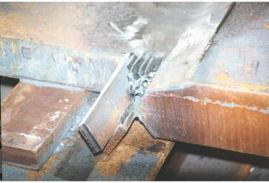
Figure 7 Photograph showing a run-off tab
