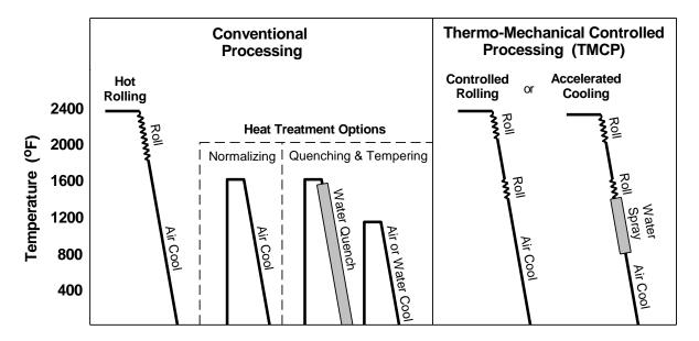
Figure 1 Relative temperature-time history for plate rolling and heat treating processes.
