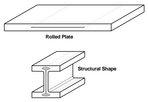
Figure 2 Segregation causes planar inclusions at the mid-thickness location of steel products.
