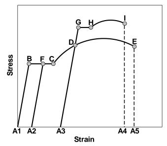
Figure 11 Stress-strain behavior showing the effects of strain hardening and strain aging.
