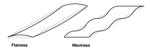
Figure 13 Illustration of plate flatness and waviness.
