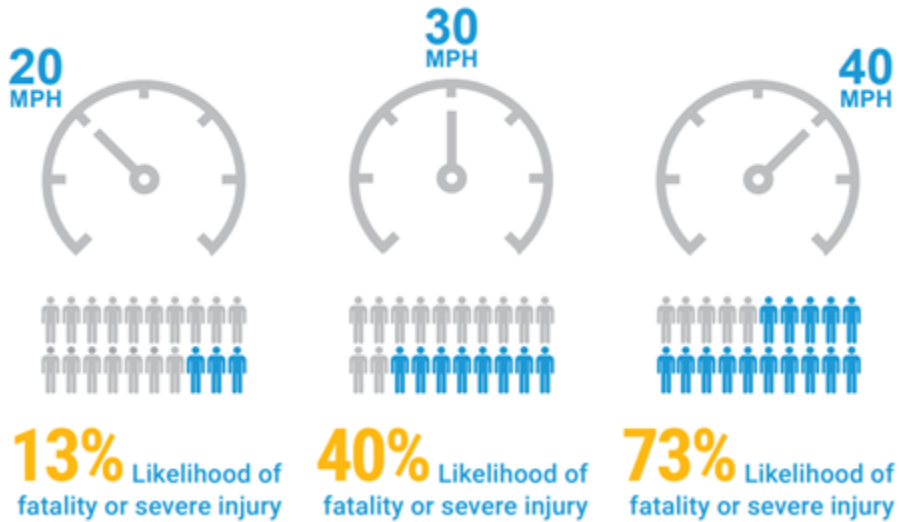
Figure 1.2 The impact speed on a pedestrian’s risk of severe injury or death. Graphic from Denver Vision Zero Action Plan (Tefft, 2013).
