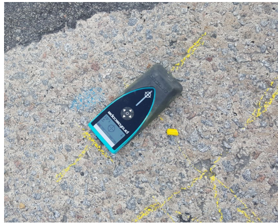
Figure 3.18: Profoscope rebar locator
