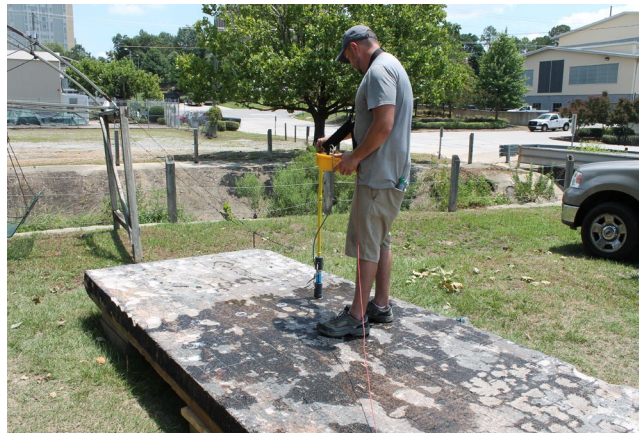
Figure 3.28: Half-cell potential testing
