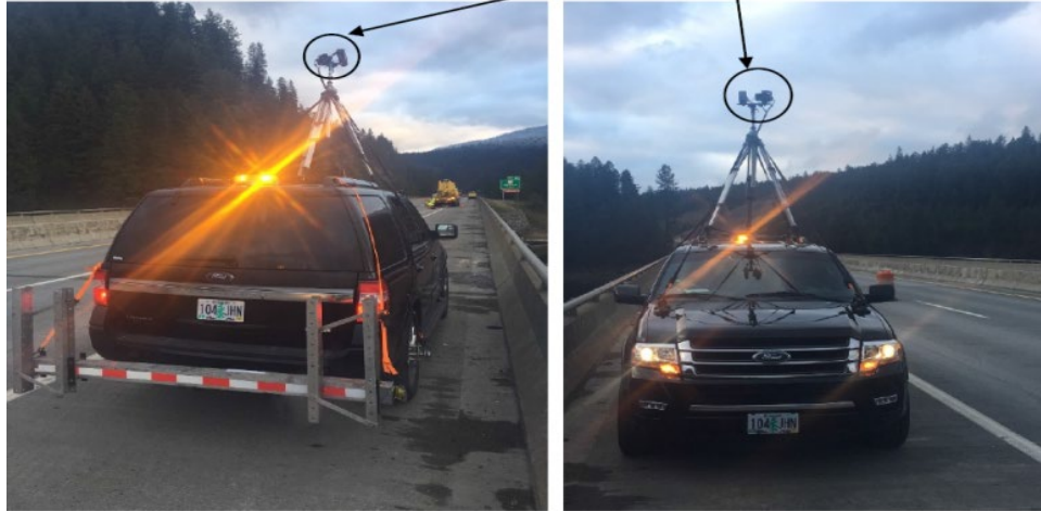
Figure 3.6: Infrared and video survey equipment (BDI and Infrasense Inc., 2017), (figure reproduced with permission)
