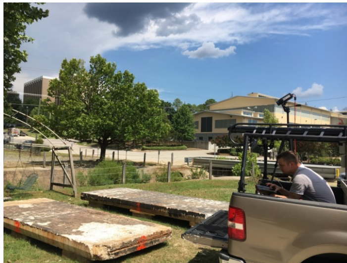
Figure 3.26: Infrared thermography scanning
