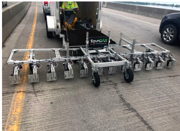
Figure 3.14: Deck acoustic response for individual solenoid impactors (BDI/Infrasense, Phase II Report, 2018) (figure reproduced with permission)
