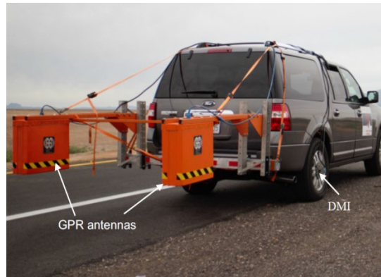
Figure 3.5: GPR survey equipment (BDI and Infrasense Inc., 2017), (figure reproduced with permission)
