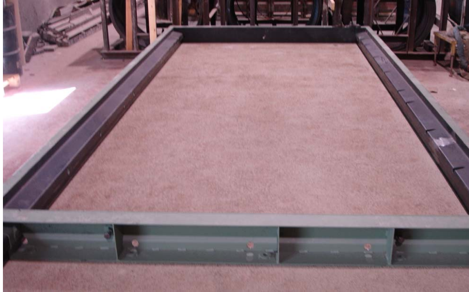
Figure 10. Photo. Casting bed and side forms.
