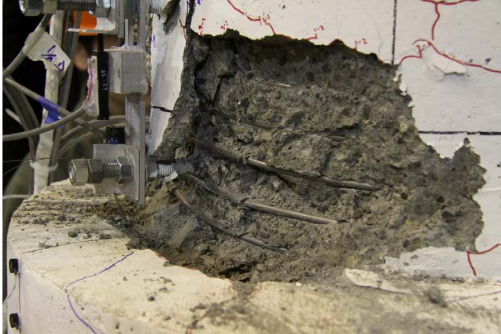
Figure 87. Photo. Specimen DS-1 – first noticeable bar buckling in the column in cycle 9-3 (6.90/-6.81 percent drift).
