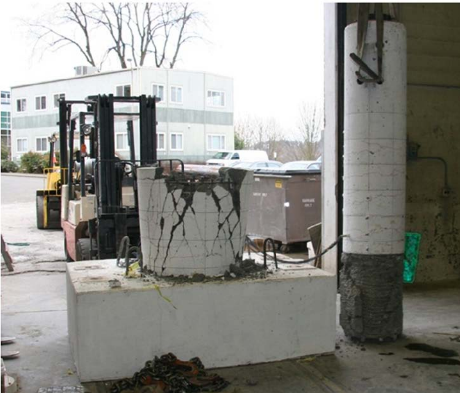
Figure 12. Photo. Specimen DS-2 after testing.
