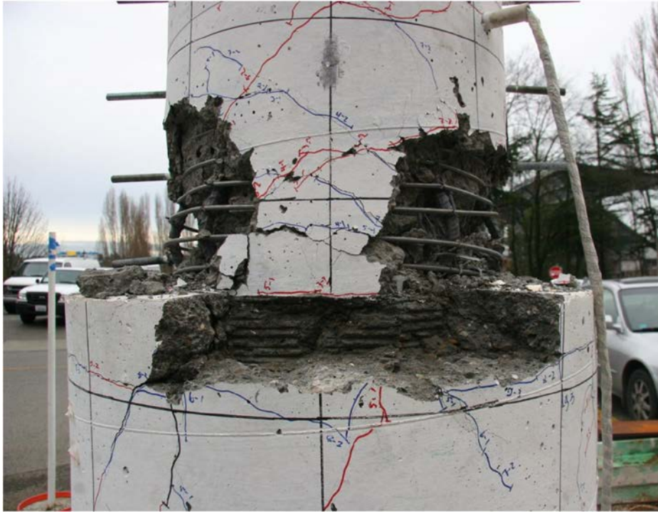
Figure 11. Photo. Specimen DS-1 after testing.
