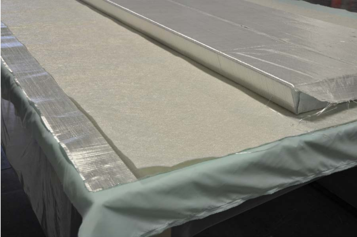
Figure 7. Photo. The panel is wrapped in glass fiber in preparation for infusion with vinyl ester resin.
