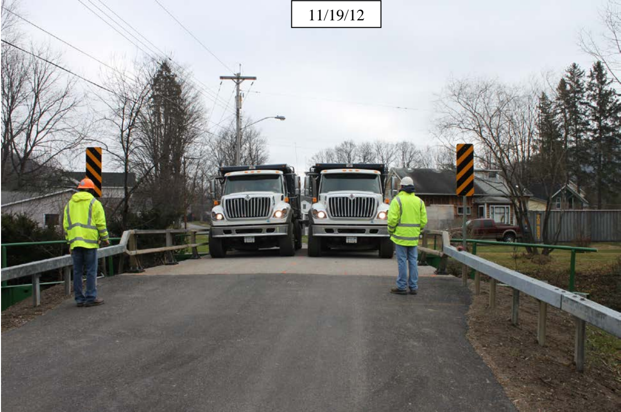
Figure 32. Photo. Load test to determine the load capacity of the bridge; not normally needed to assess the deck.
