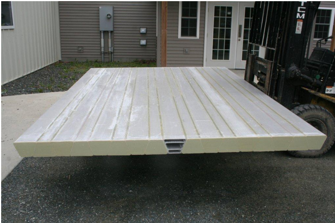
Figure 6. Photo. Panel ends are capped and radii between tubes filled with thixotropic resin.
