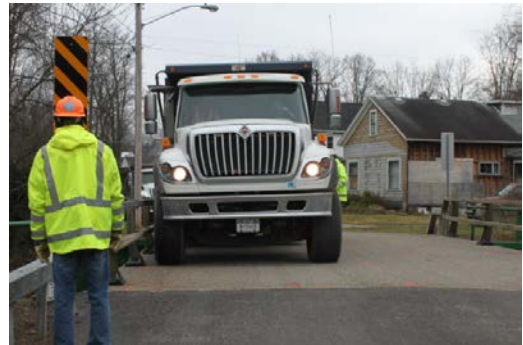
d) Photograph of truck on load path BN, load case 2
