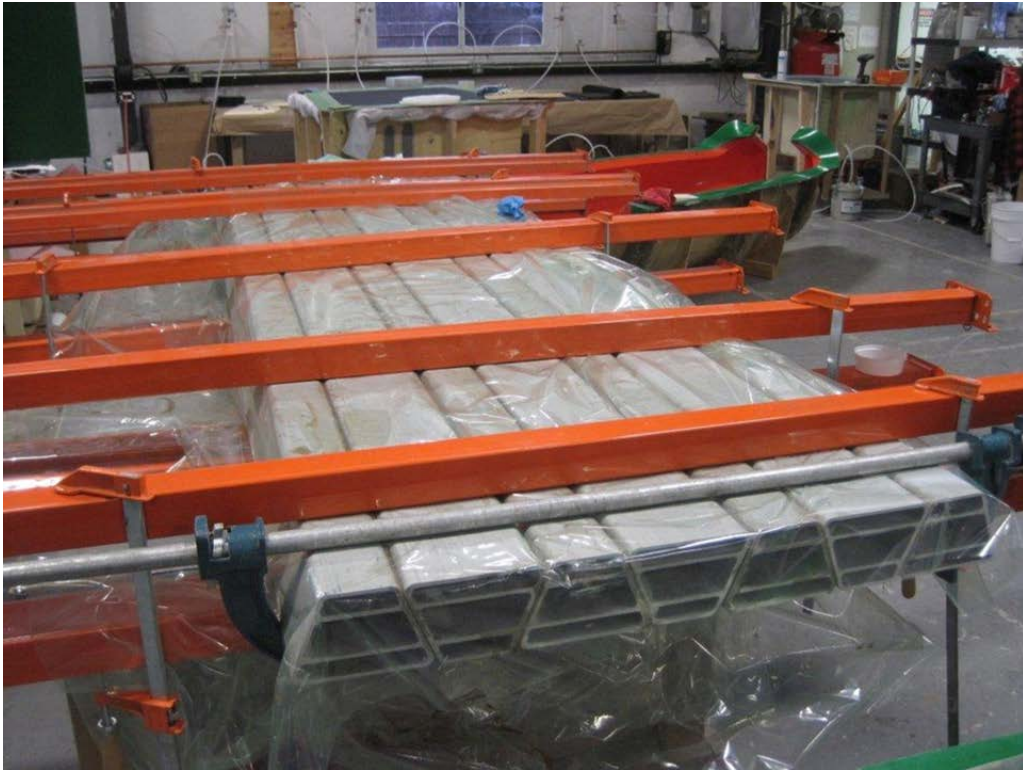
Figure 5. Photo. Tube subcomponents are bonded together with adhesive to form a panel.
