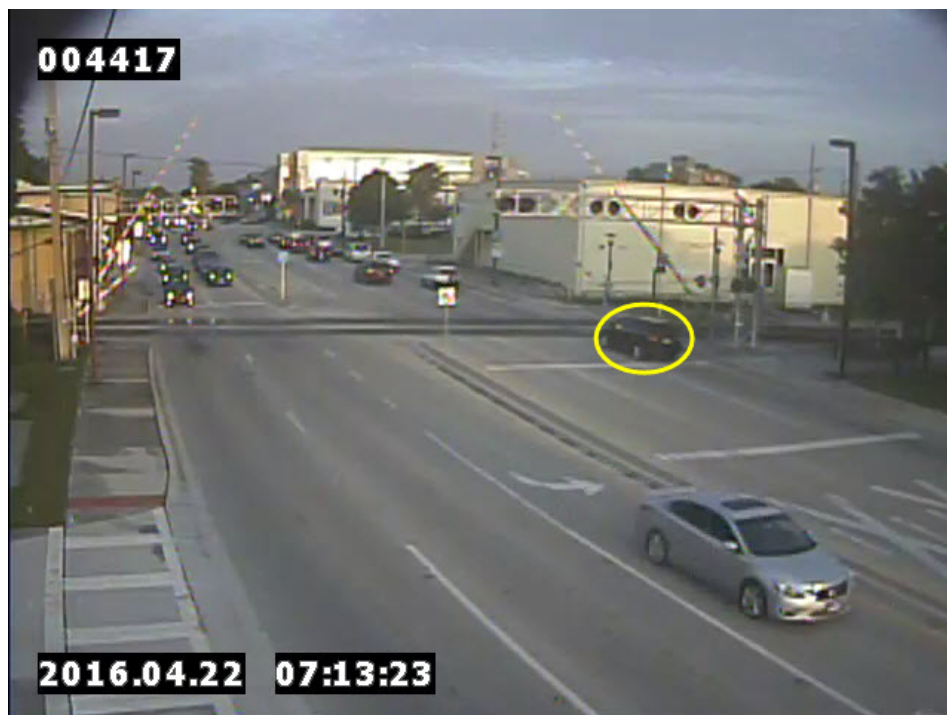
Figure 22. Example of Type II Violation in Westbound Direction (Yellow Circle)
