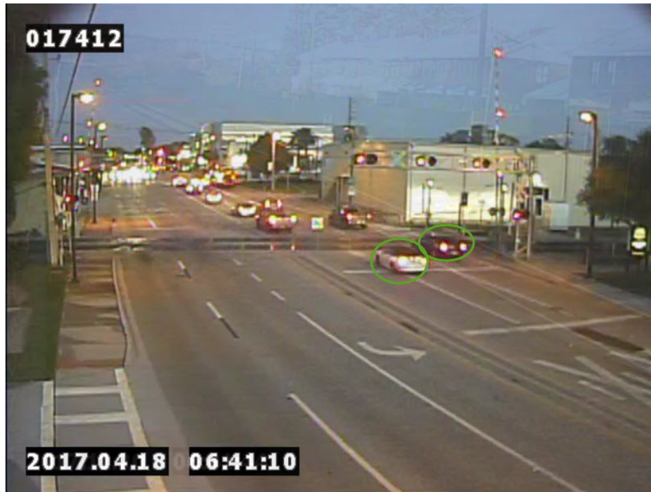
Figure 20. Example of Type I Violations in Westbound Direction (Green Circles)
