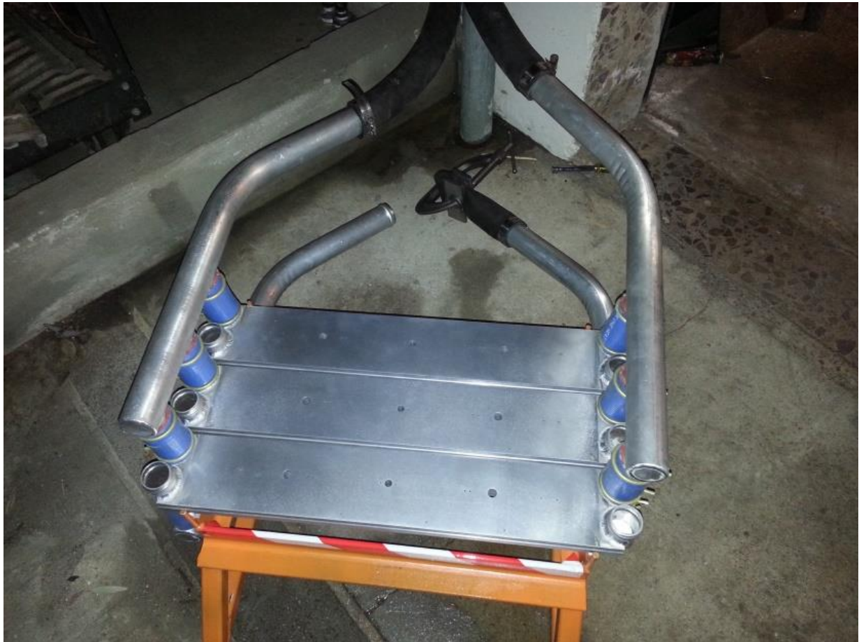
Figure 72. Leak testing cold-side heat exchangers
