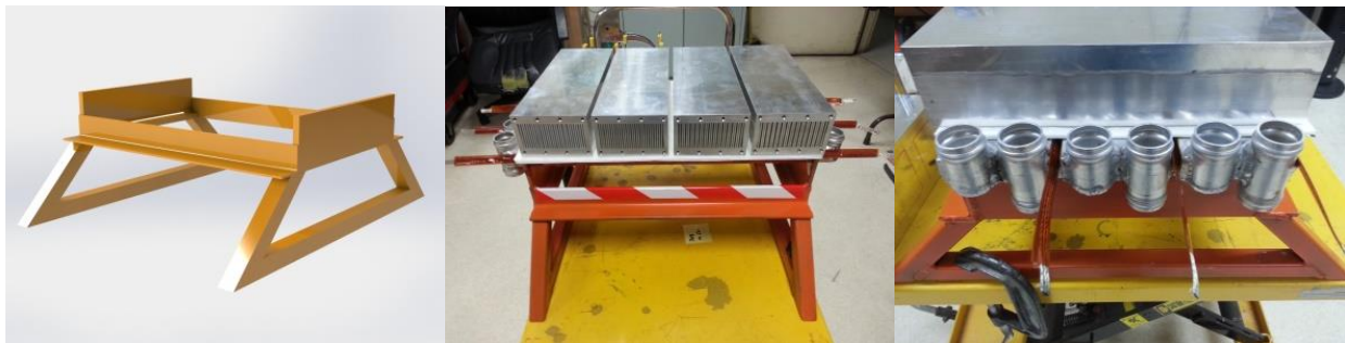
Figure 70. Assembly Jig and first layer of heat exchangers, modules and insulation
