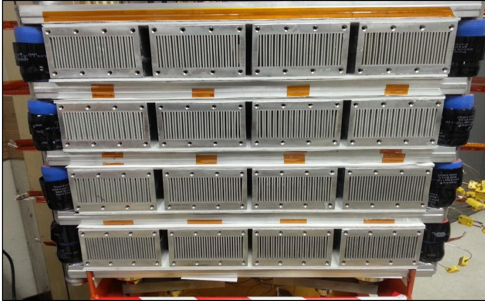
Figure 10. Sectional layers of the TEG allow passage of the engine exhaust gases.
