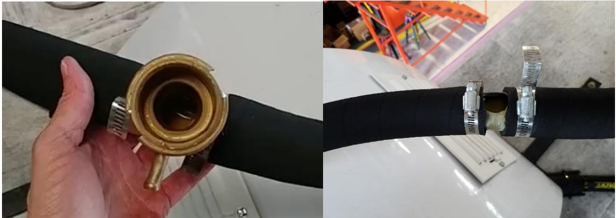
Figure 59, 60. Before and After Coolant Filler Neck
