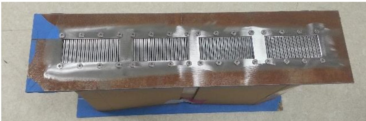
Figure 26. Sandblasting Mask for Burr Removal
