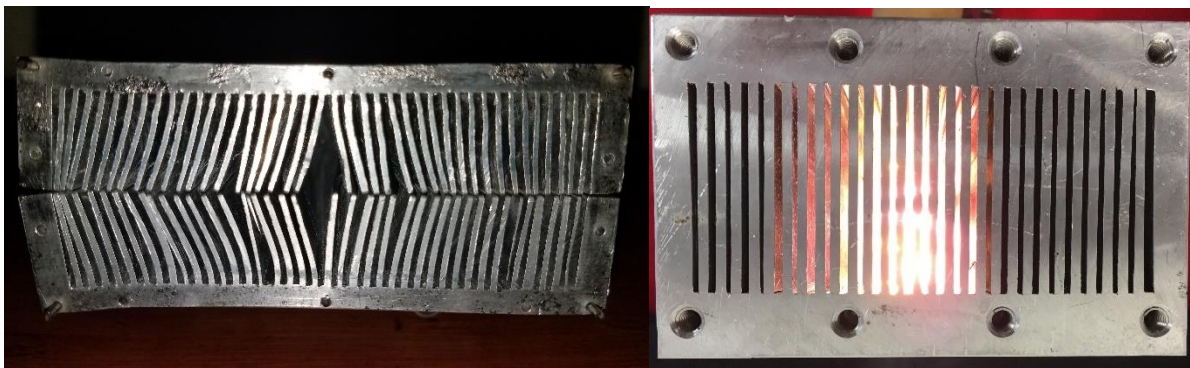
Figures 22, 23. Damaged Prototype HXh vs Final Design HXh
