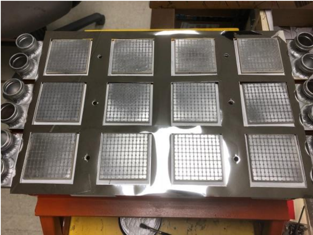
Figure 71. Aluminized Kapton layer of MLI
