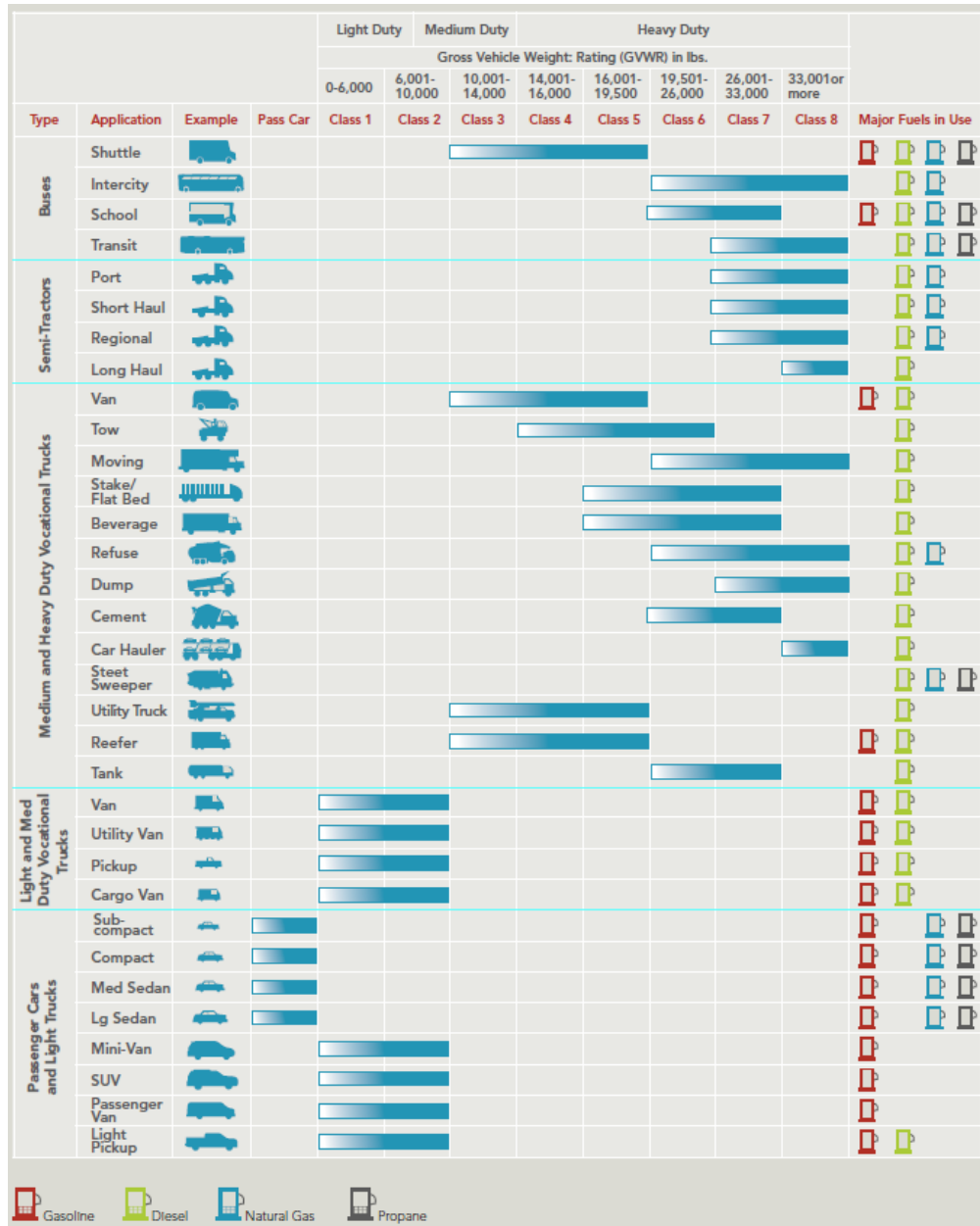
Figure 4: U.S. DOT Vehicle Classes and Fuels in Use for Various Transportation Applications
