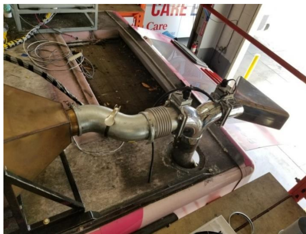
Figure 42. Diverter Valve Mounted to Bus Exhaust
