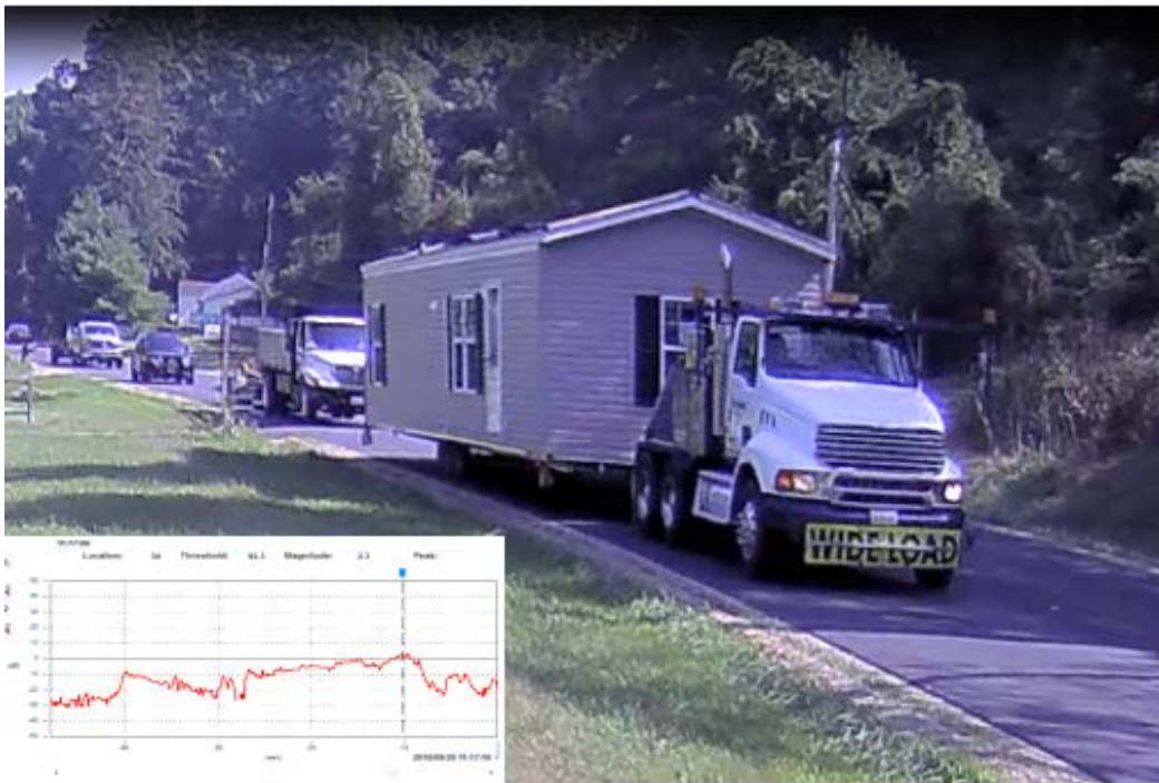
Figure 17. BCADS Interference Occurred at Various Locations along the Cable System Due to Encroachment of Oversized Vehicles into the Sensing Area. BCADS = Buried cable animal detection system.
