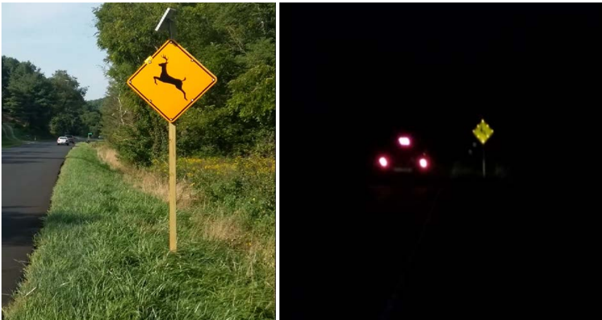
Figure 16. Warning Sign Flashing During the Day (LEDs Appear as White Dots) and at Night. LED = light emitting diode.
