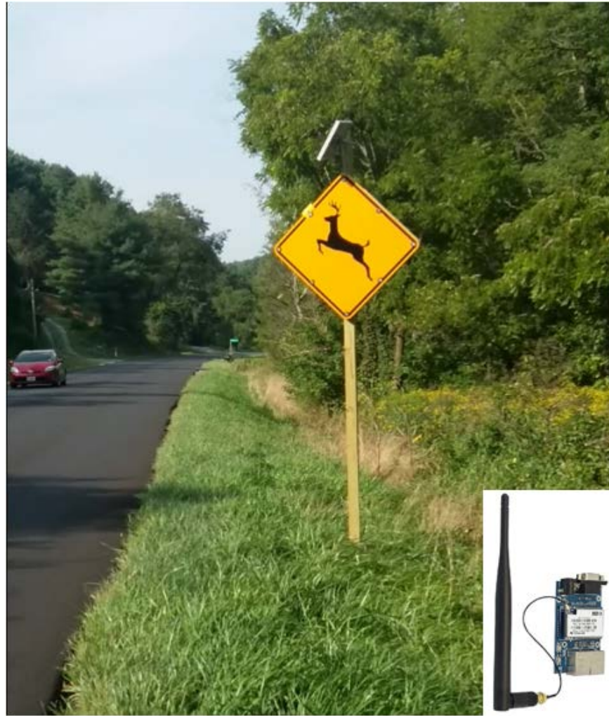
Figure 13. Deer Warning Sign with Flashing LEDs Installed on Riner Rd. Wireless Transceivers Shown at Bottom Right. LED = light emitting diode.
