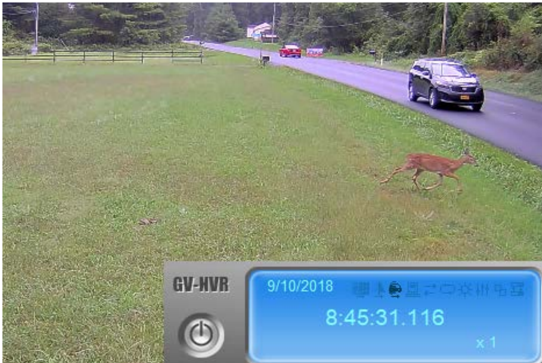
Figure 15. Example of Valid Animal Detection Event Showing Event Date and Time Corresponding to the Declared Alarm in the Event Log Pane (Figure 14).
