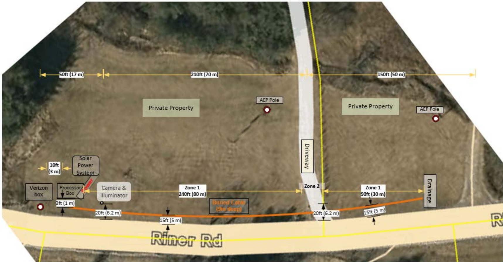
Figure 4. Plan View of the Test Site Showing the Location of the BCADS Installation and Respective Detection Zones. BCADS = buried cable animal detection system.
