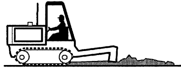
1. Rip and break existing pavement
