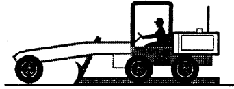
3. Windrow Existing Asphalt Bound Materials
