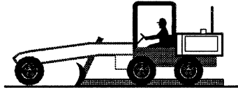
3. Windrow Existing Asphalt Bound Materials
