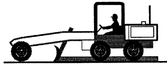
3. Windrow Existing Asphalt Bound Materials
