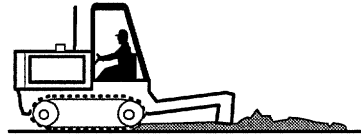
1. Rip and break existing pavement
