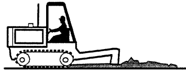
1. Rip and break existing pavement
