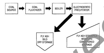
Figure 1. Fossil fuel power plant schematic.
