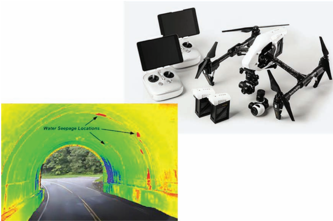
Figure 5.15 Infrared thermography using drones. (Images from http://www.flir.com/suas/aerial-thermal-imaging-kits/ .)
