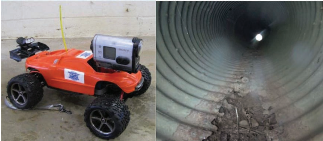
Figure 6.6 The HIVE camera unit and image taken by it. (Source: http://dot.state.mn.us/research/reports/2017/201716.pdf .)
