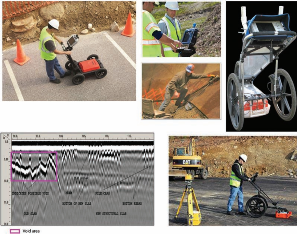
Figure 5.8 Ground penetrating radar: equipment, in-situ operation, and application output graph showing a detected void. (Images from envirophysics.com & alphageofisica.com.br .)
