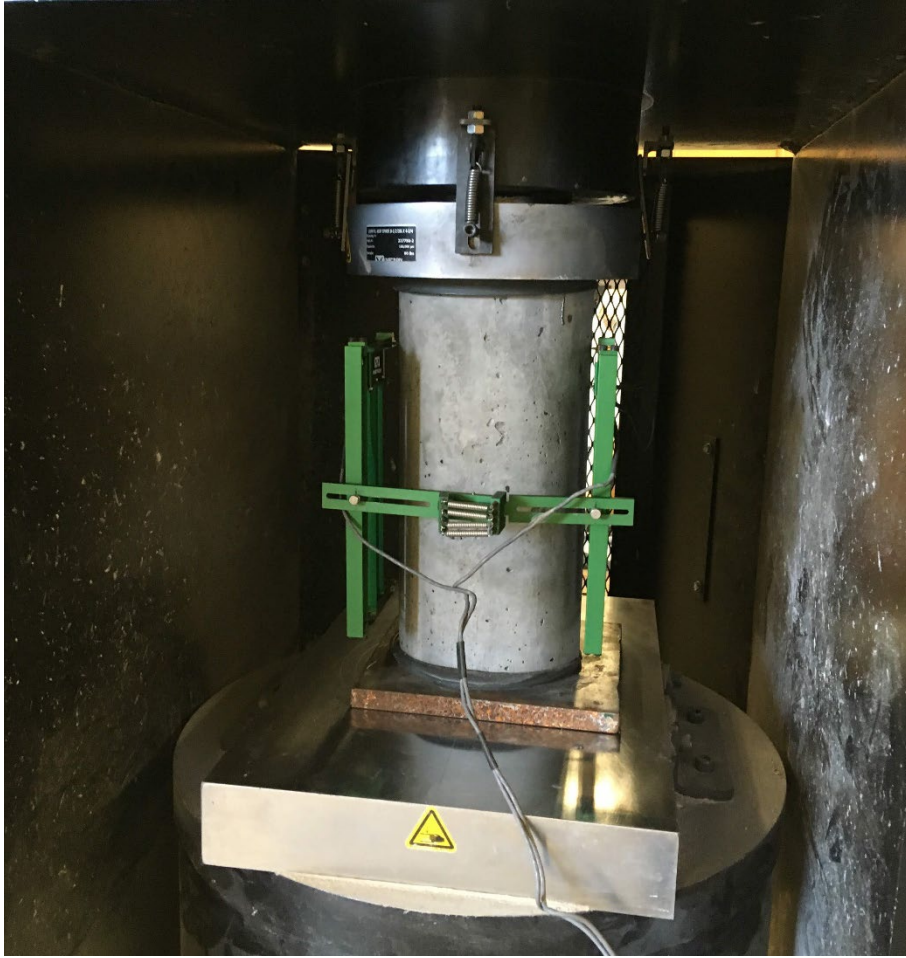
Figure 3.11 Compressive strength testing setup
