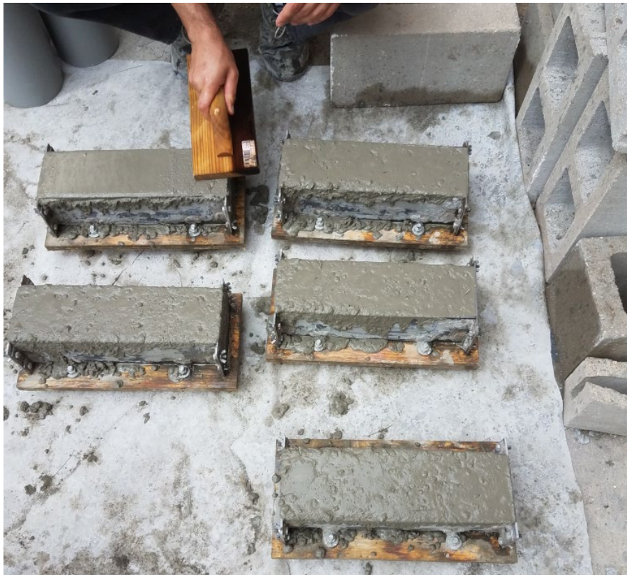
Figure 3.6 Finishing using a wooden trowel
