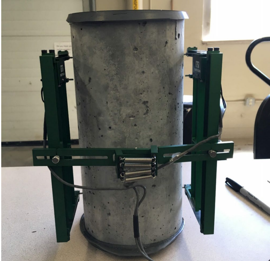
Figure 3.10 8" Extensometer used to measure the compressive strain of a concrete cylinder during testing, according to ASTM C39
