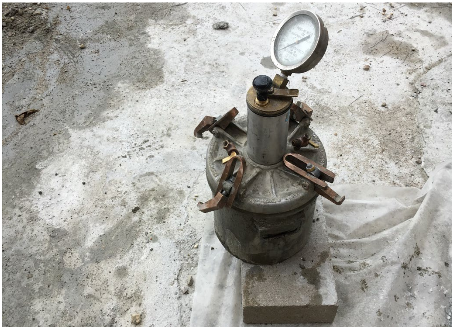
Figure 3.9 Air meter used to determine the concrete's air content, according to ASTM C231
