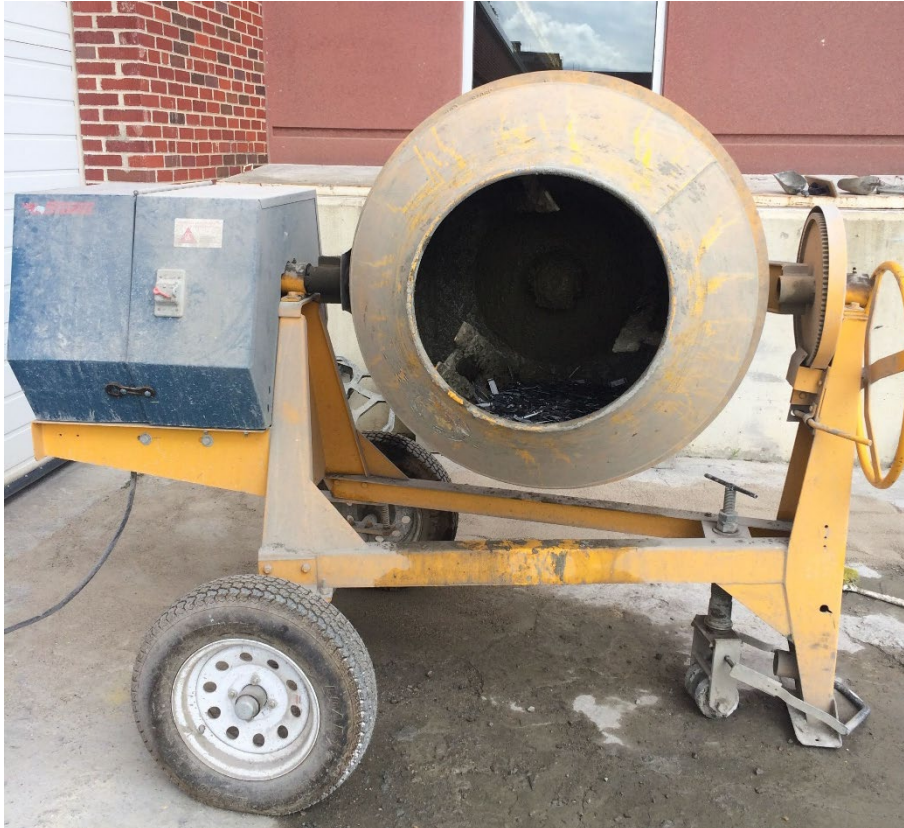
Figure 3.1 ½-cubic-yard capacity concrete drum mixer
