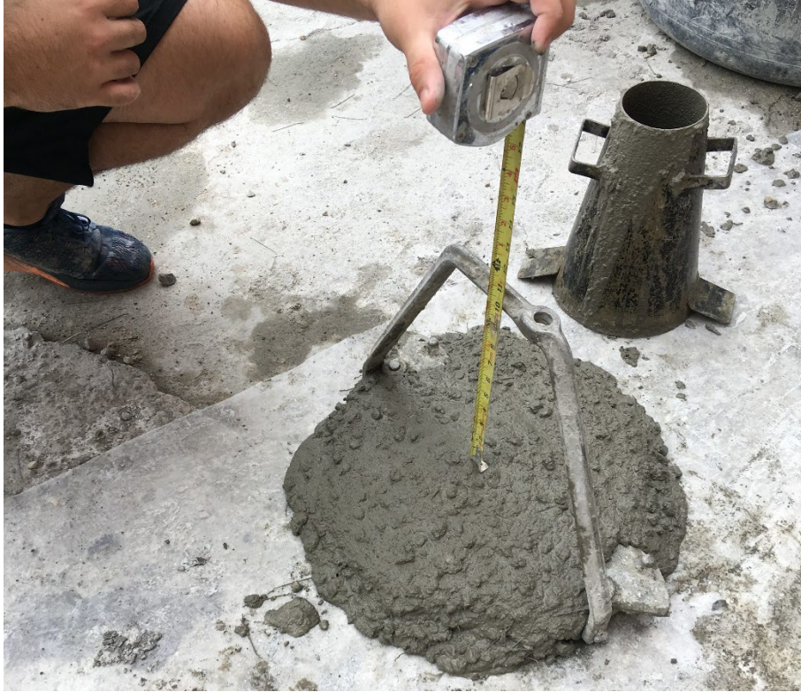
Figure 3.8 Measurement of the concrete slump, according to ASTM C143
