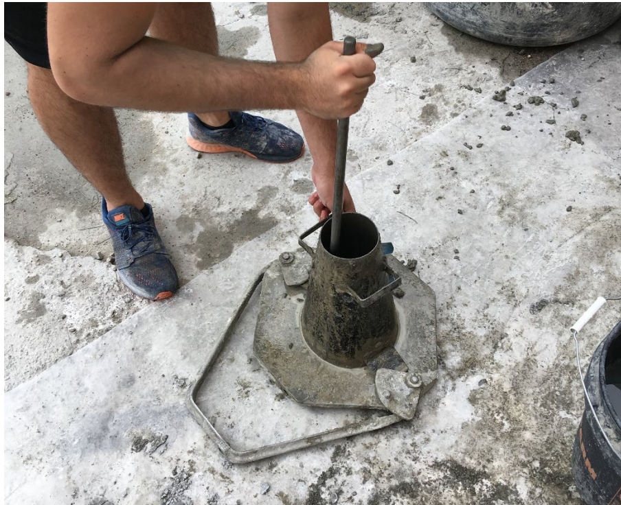
Figure 3.3 Rodding during a concrete slump test
