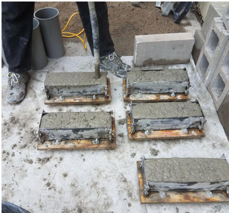
Figure 3.4 Hand-held spud vibrator in use
