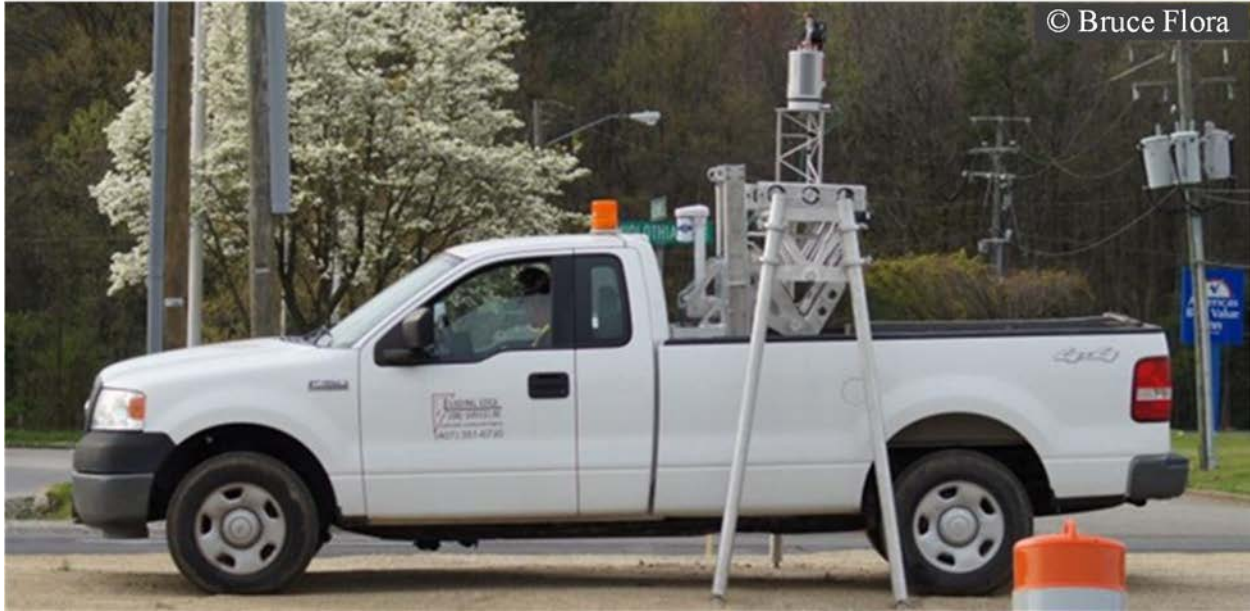
Figure 33: Photo. TopoLIFT® system collecting static lidar survey.
