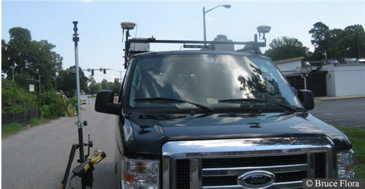
Figure 31: Photo. Truck with GNSS receivers for rolling survey.
