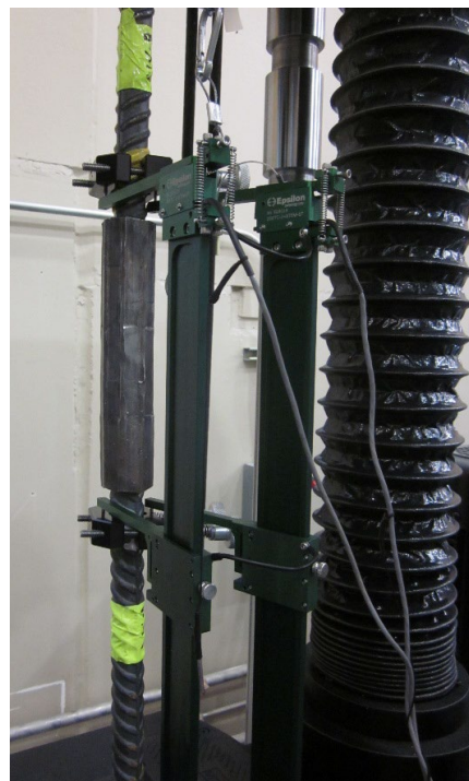
(b) Device with coupler extensometer
