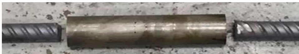
Figure 3.10 Preparation of Erico threaded couplers
