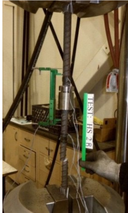
(b) Device with extensometer (Haber et al., 2015)
