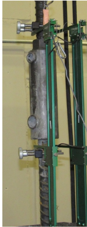
b. Coupler extensometer
