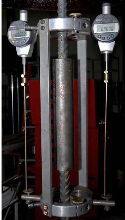
(a) Device with dial indicators (California Test 670)
