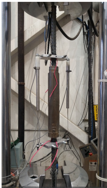
(c) Device with two LVDTs (NCHRP 12-105)
