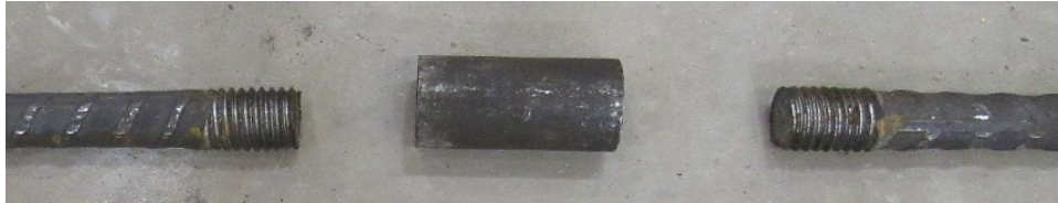
Figure 2.3 One sample of threaded couplers
