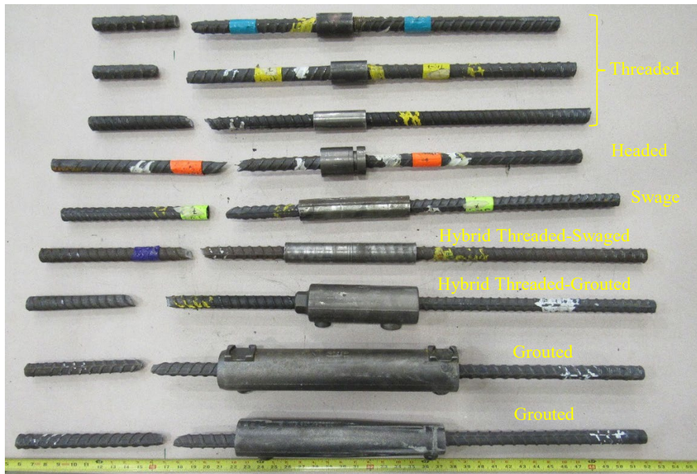
Figure 2.1 Different mechanical bar splice products and types
