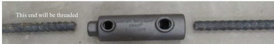
a. Threaded-grouted hybrid coupler
