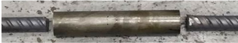
Figure 2.6 One sample of swaged couplers
