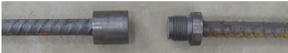
Figure 2.4 One sample of headed reinforcement couplers
