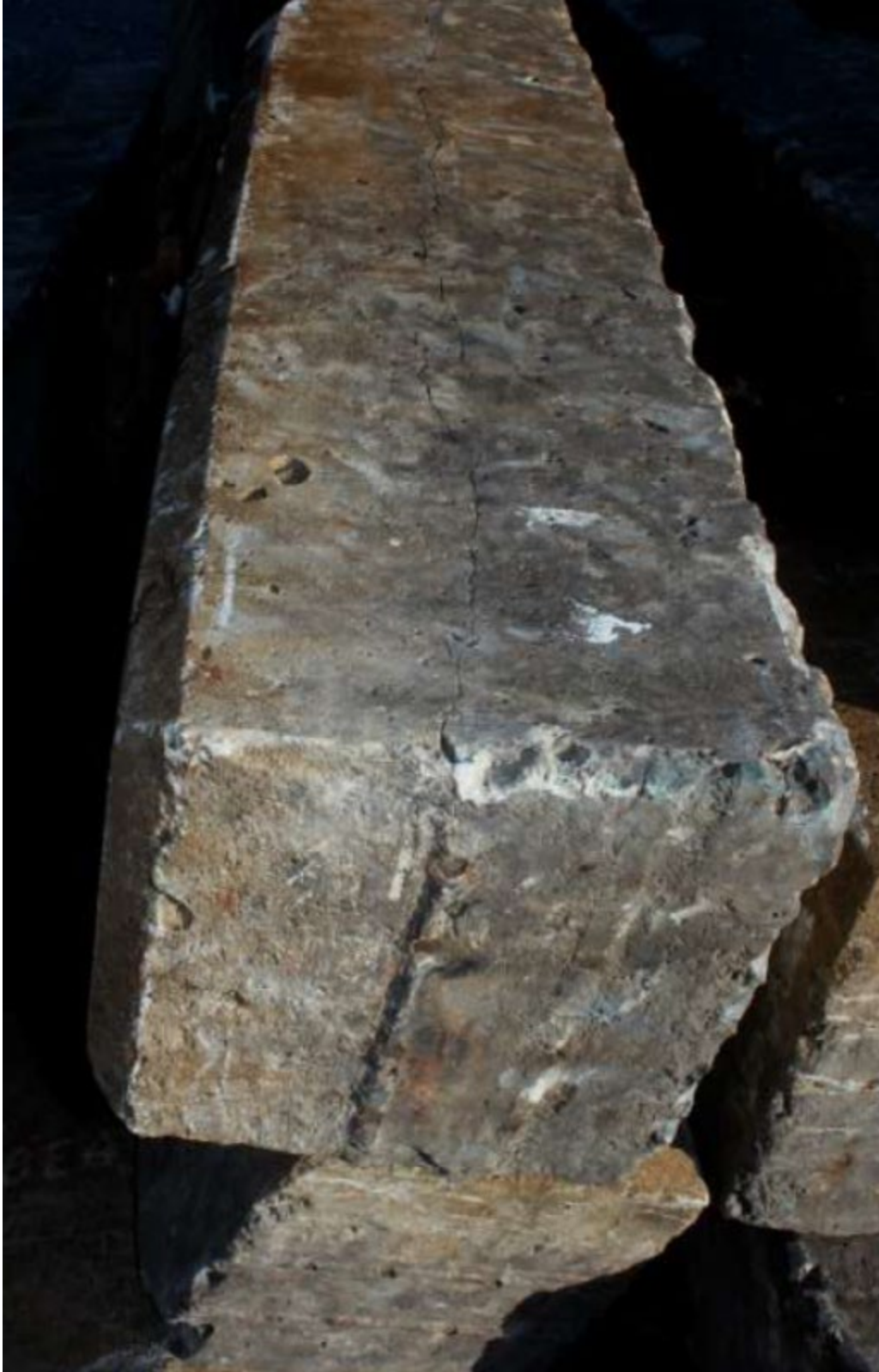
Figure F-9: Longitudinal splitting cracking seen in tie in stack 1, Boneyard #2
