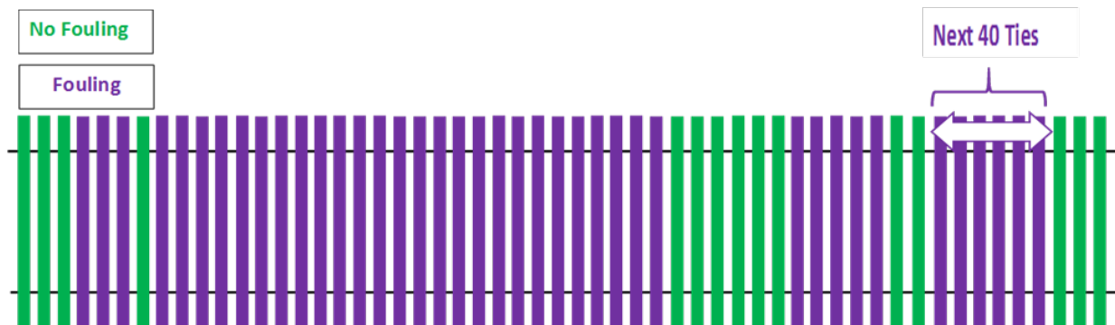
Figure E-12: Schematic view of fouling, Tangent #3
