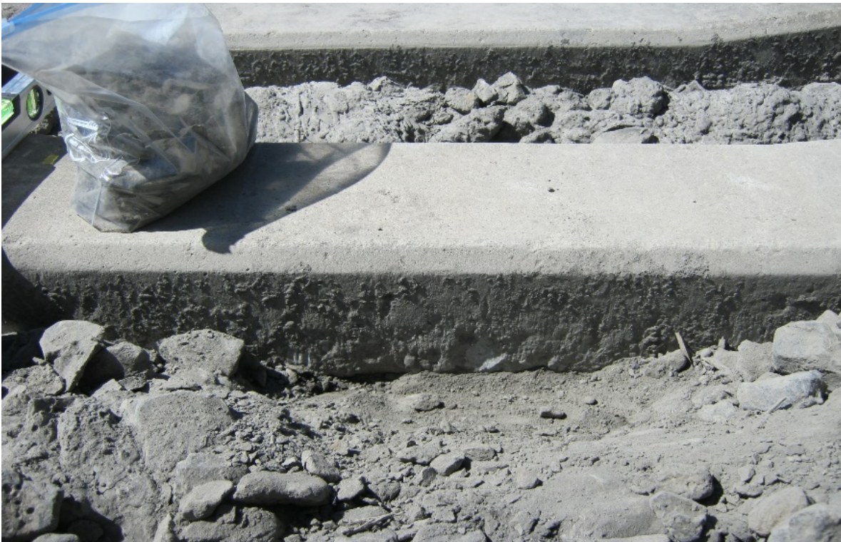
Figure B-5: Sample collection from ballast at depth of tie bottom, Switch #1
