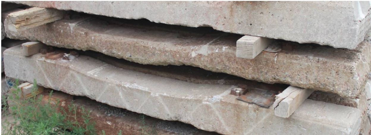
Figure F-2: Tie with significant non-uniform abrasion damage, Boneyard #1
