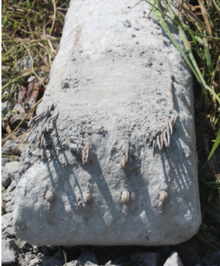
Figure 3-15: Bottom of a tie made with limestone coarse aggregates found with abrasion damage on the side of the road
