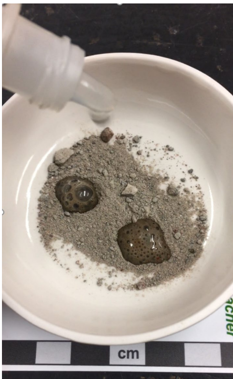
Figure 2-3: Ballast fines sample that was carbonaceous and reacted with the addition of hydrochloric acid
