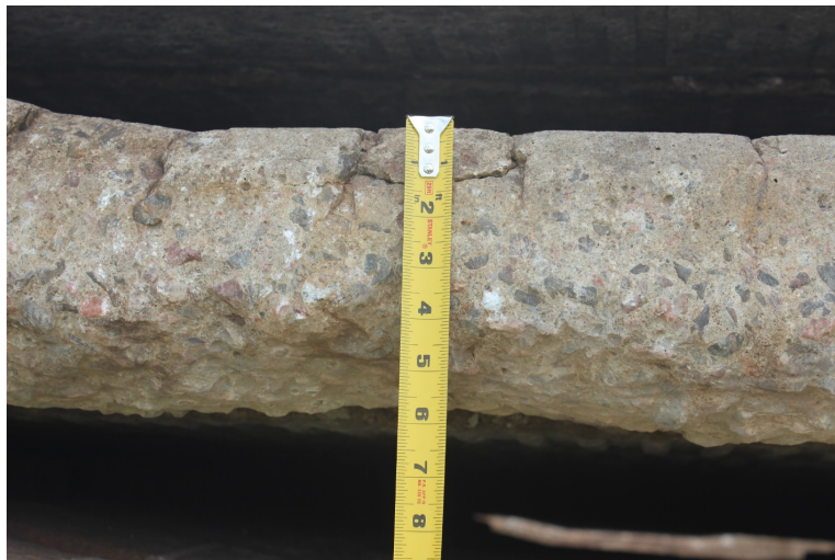
Figure 3-16: Tie made from hard siliceous aggregates in boneyard with significant abrasion damage
