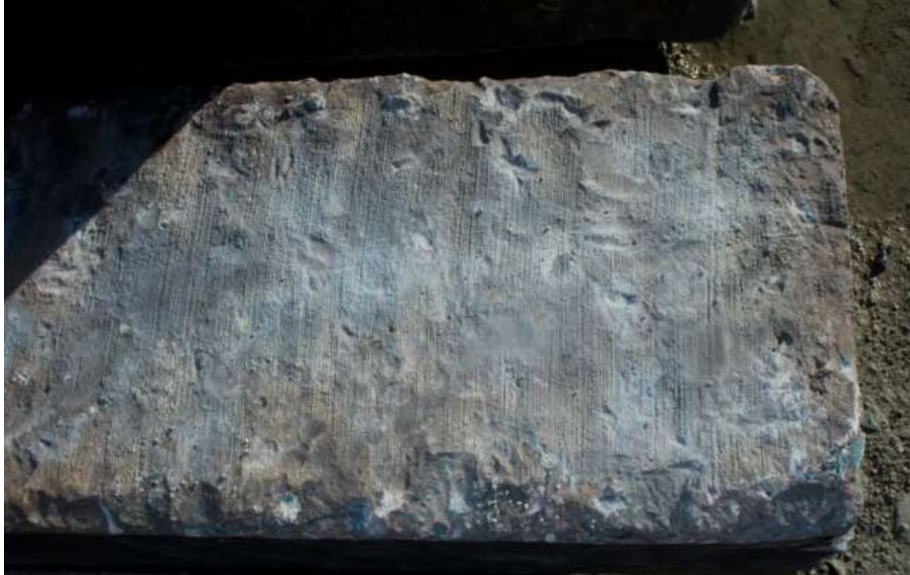
Figure F-7: Broom finish still visible on bottom of many ties in stack 1, Boneyard #2
