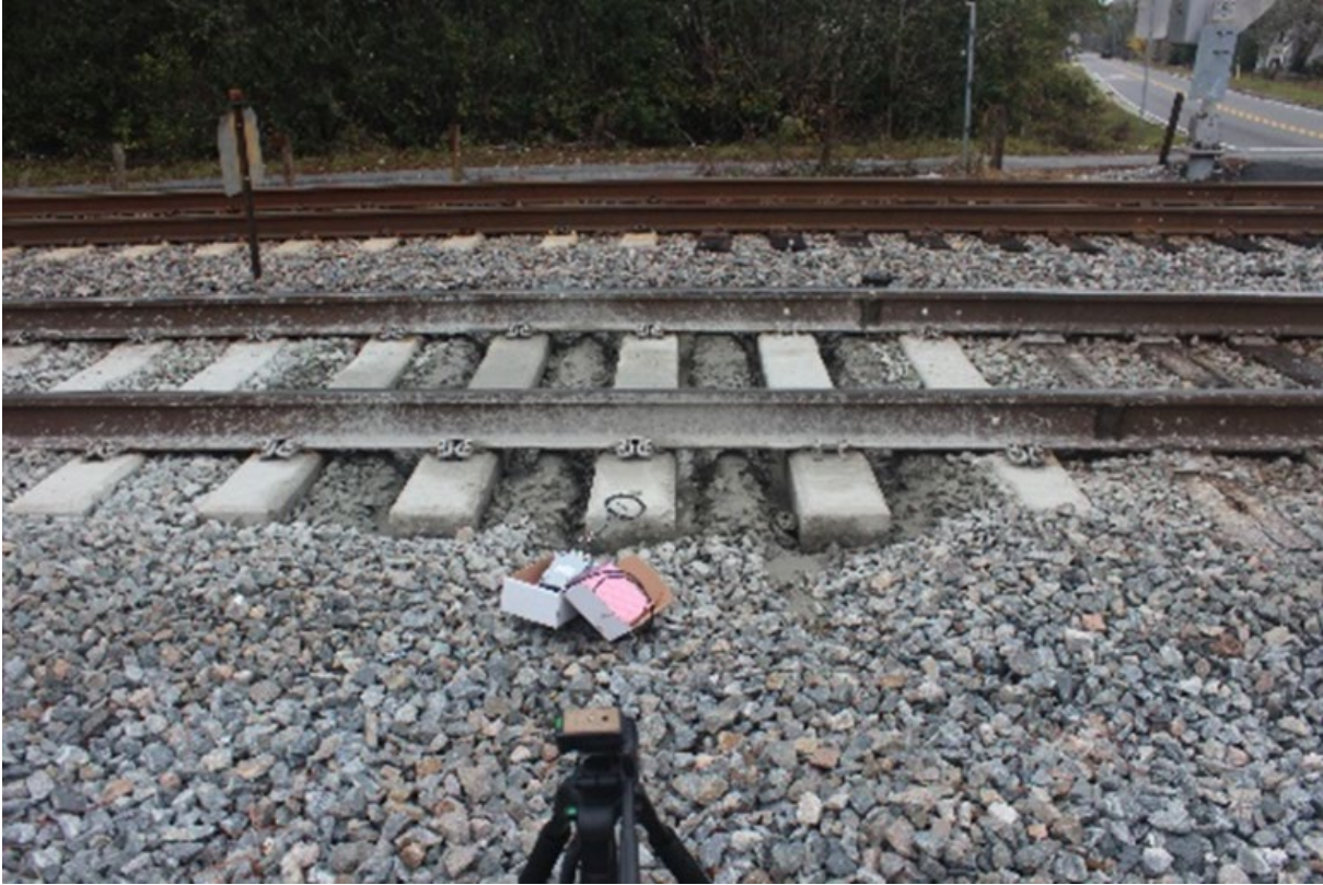
Figure C-31: Tie acceleration and deflection were measured using an accelerometer and high-resolution camera, Crossing #5
