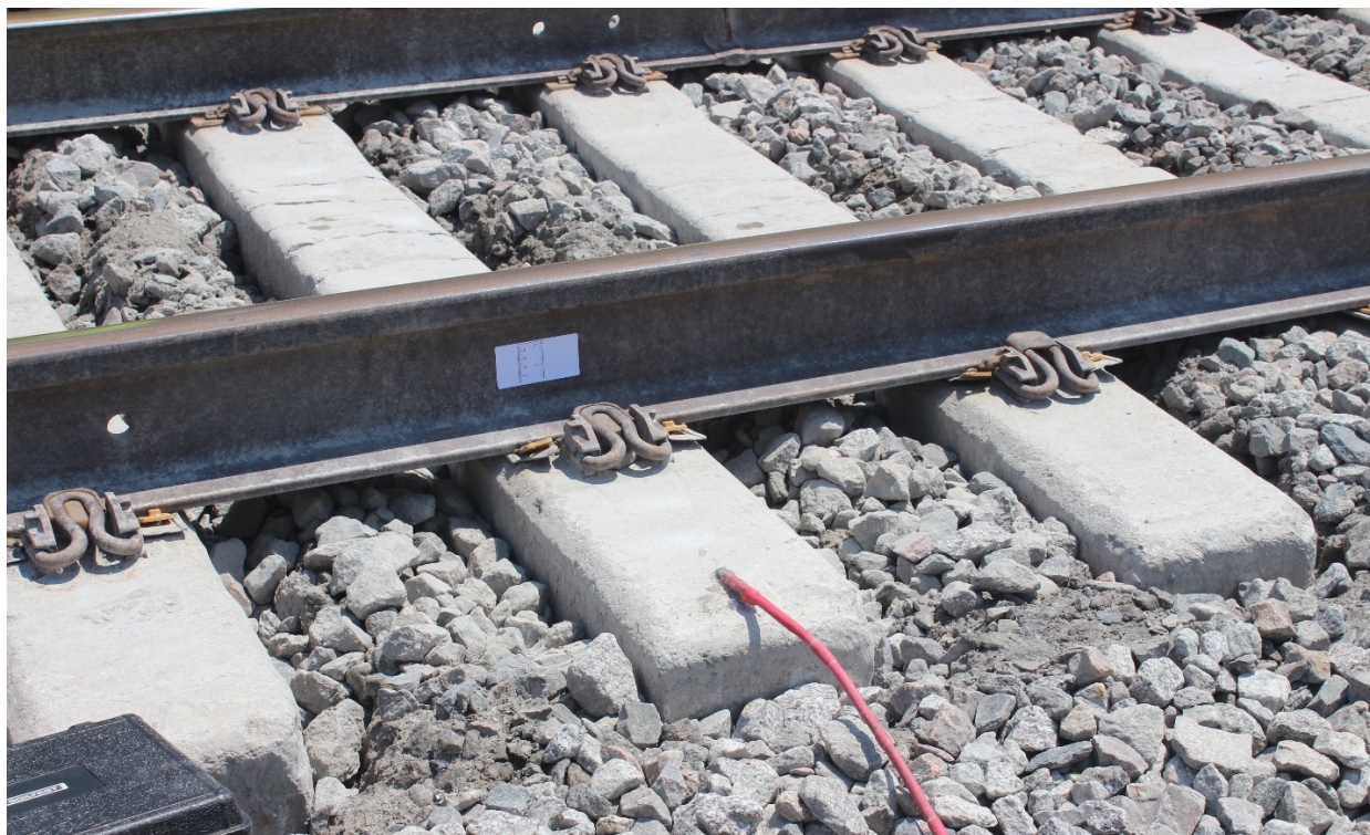
Figure B-19: Accelerometer placed on tie to measure acceleration in three directions, Signal #2
