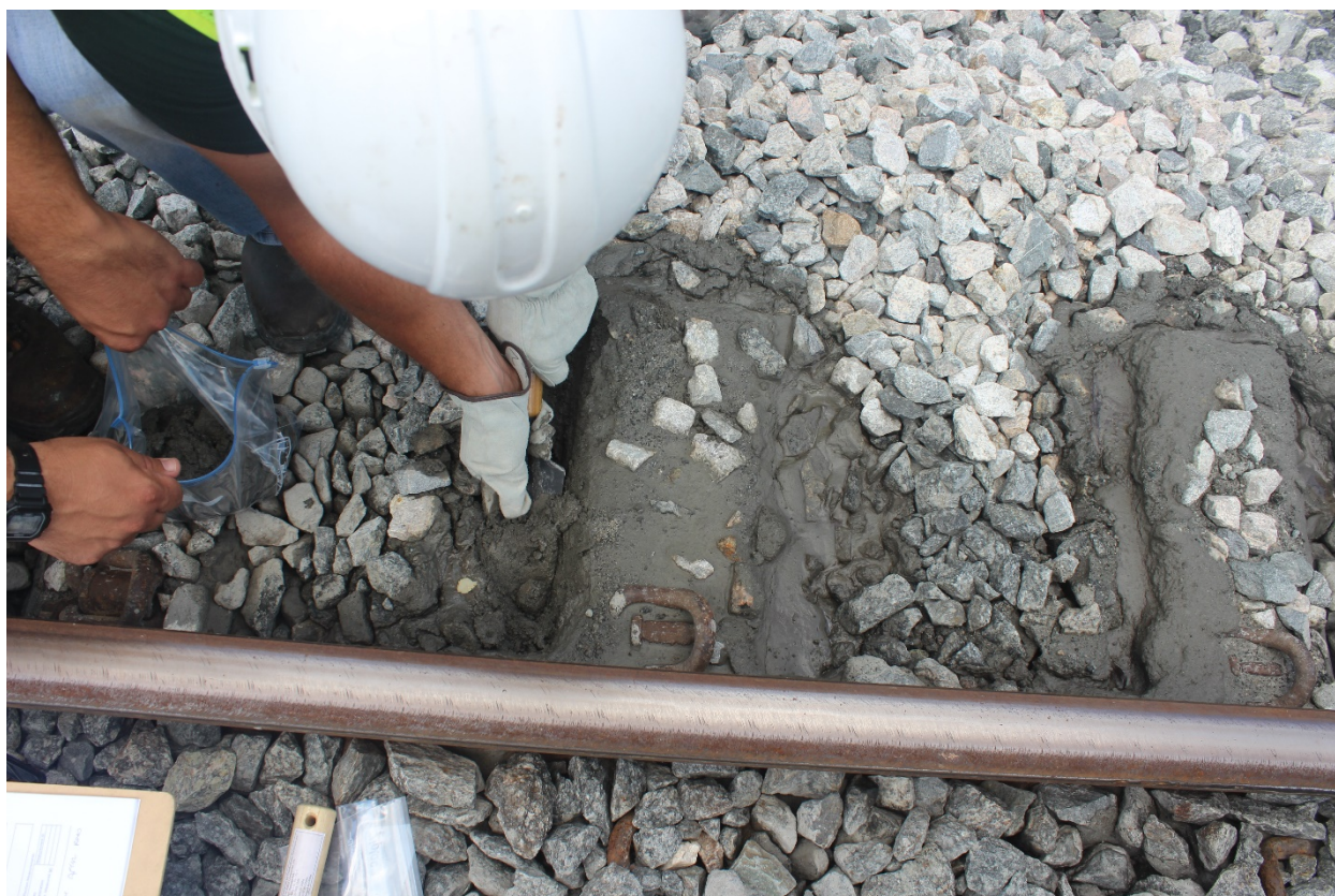
Figure C-49: Ballast sample collection, Crossing #8
