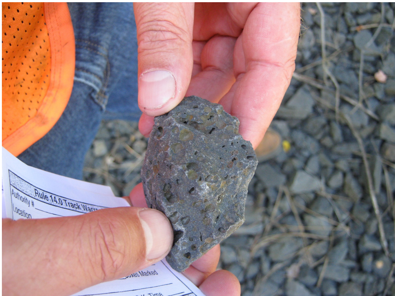
Figure C-8: Close-up picture of vesicular basalt ballast, Crossing #1
