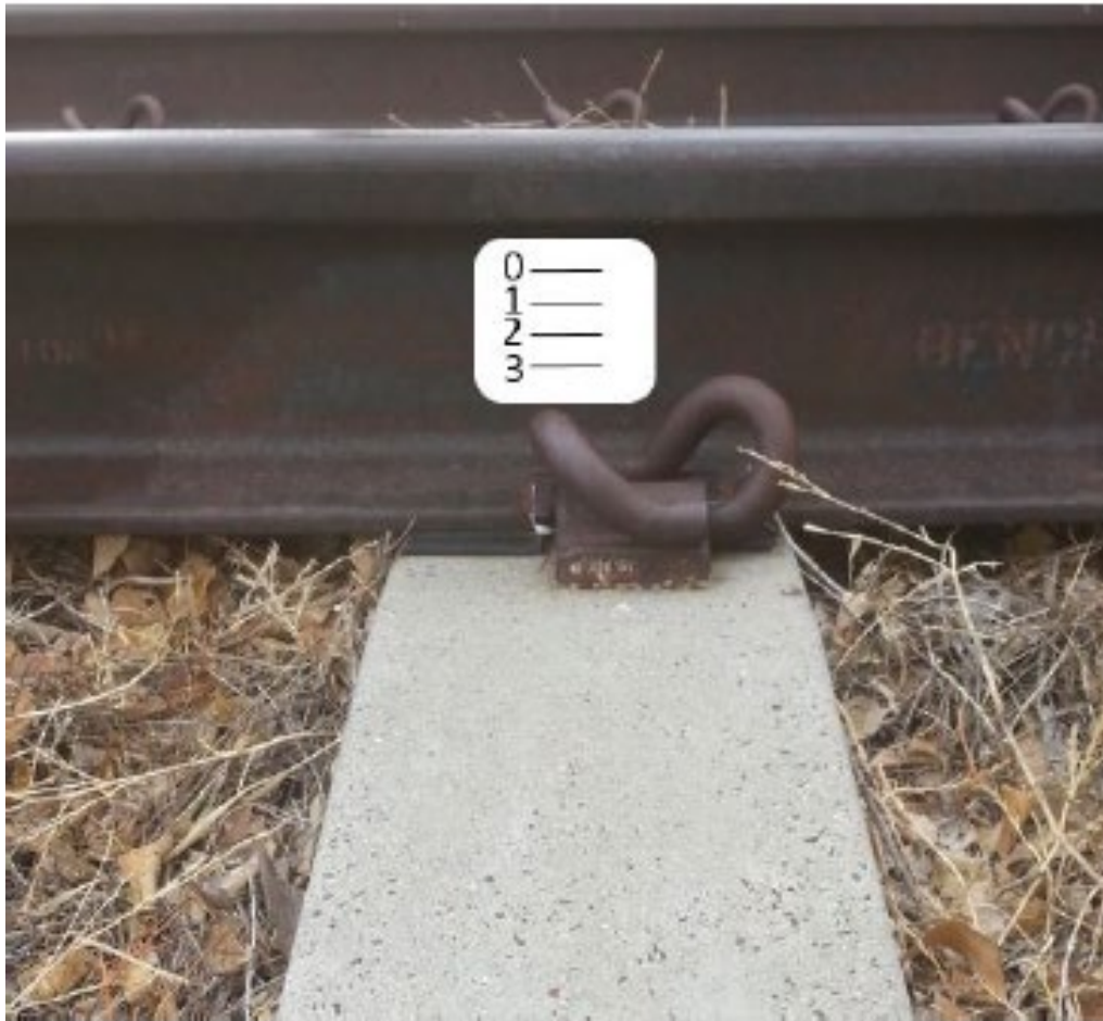
Figure 2-4: Schematic of rail with attached sticker to measure the deflection as the train passes
