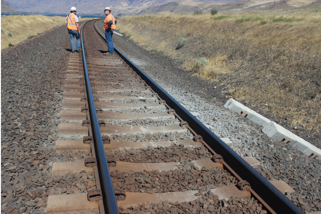
Figure D-14: Gray-colored fouling present on ballast, Curve #3
