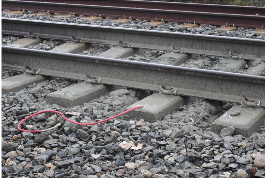
Figure A-31: Accelerometer attached to the side of the tie, Bridge Approach #3
