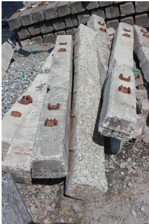
Figure F-12: Tie with some abrasion damage, Boneyard #3
