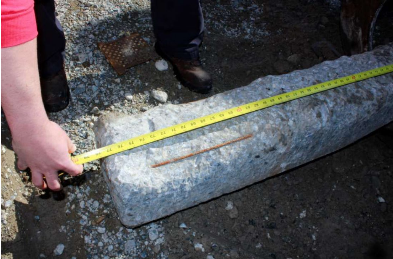
Figure F-10: Tie with severe abrasion wear in stack 2, Boneyard #2
