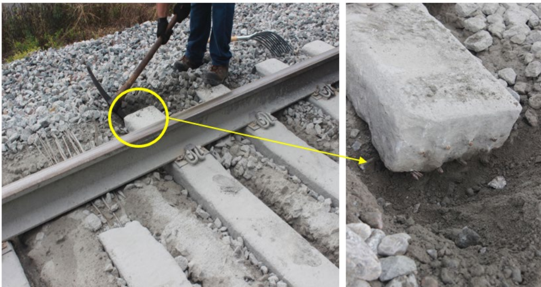
Figure C-19: Samples taken from subgrade and ballast, Crossing #3
