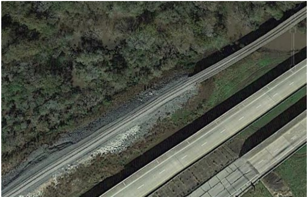
Figure A-19: Bridge Approach #1 with excessive pumping from Google Earth
