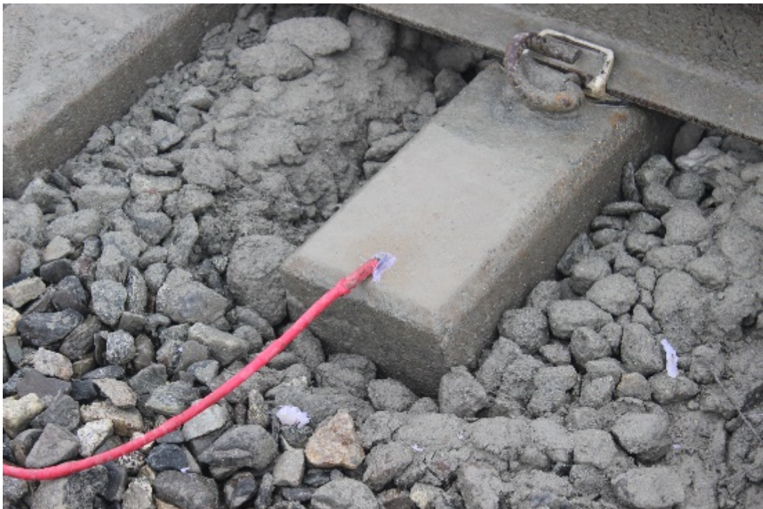
Figure 2-6: Accelerometer attached to the end of a tie before a train pass
