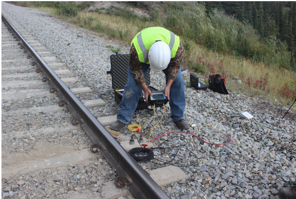
Figure E-50: UPV testing, Tangent #9
