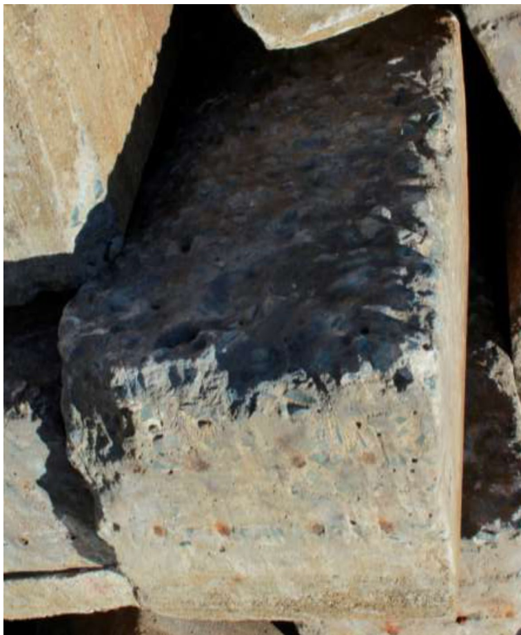
Figure F-8: Minor abrasion present in tie in stack 1, Boneyard #2
