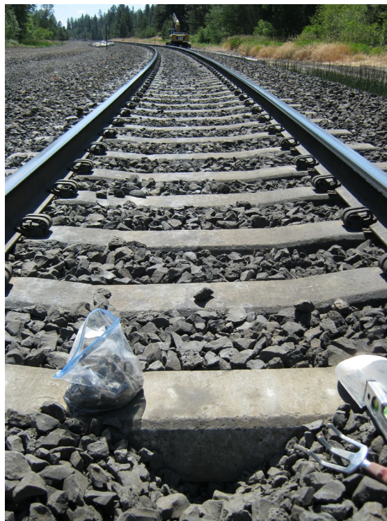
Figure B-9: Ballast samples collected from the middle of the track, Signal #1
