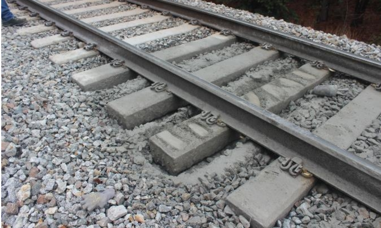
Figure E-28: Preparation of tie for Schmidt hammer testing, Tangent #6
