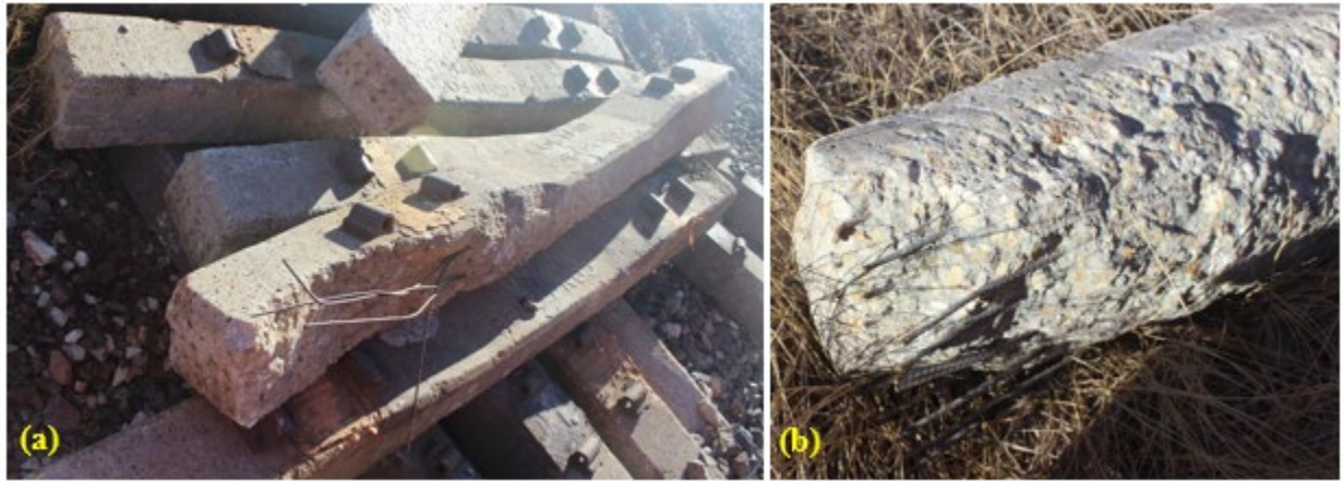
Figure F-21: Highly abraded concrete tie, Boneyard #6
