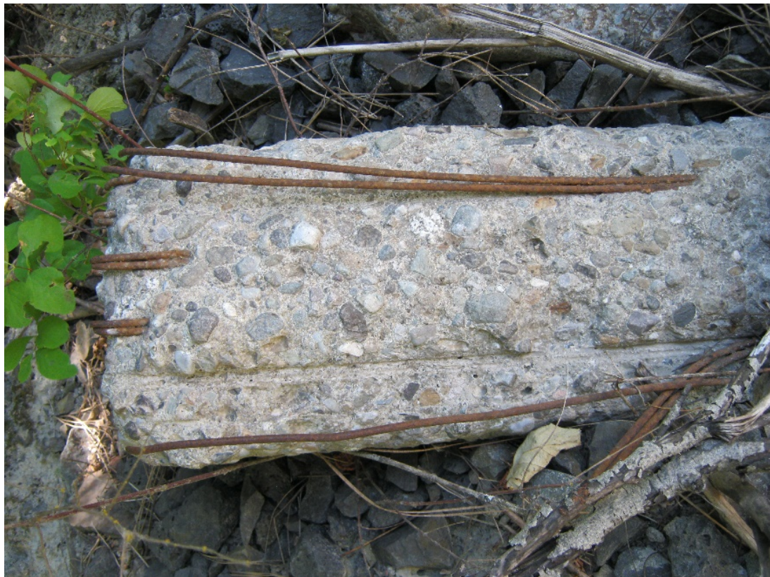
Figure C-5: Tie with abrasion removed from track, Crossing #1
