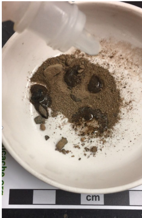
Figure 2-2: Ballast fines sample that was not carbonaceous and did not react with the addition of hydrochloric acid
