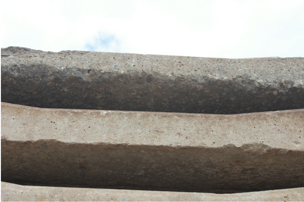
Figure F-3: Picture of tie bottom with severe abrasion damage, Boneyard #1
