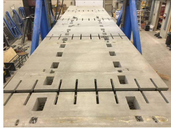
Figure 4.10 Installation for Full-depth Deck Panels on Precast Girders
