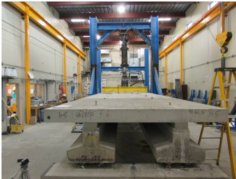
Figure 4.16 Ultimate Test Setup for the Precast Bridge Specimen
