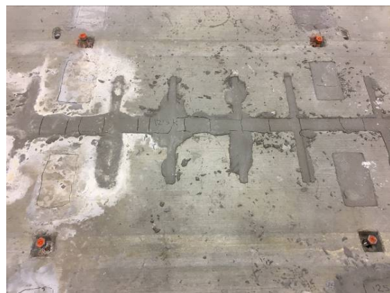
(b) Latex Modified Concrete at 650,000 Cycle
