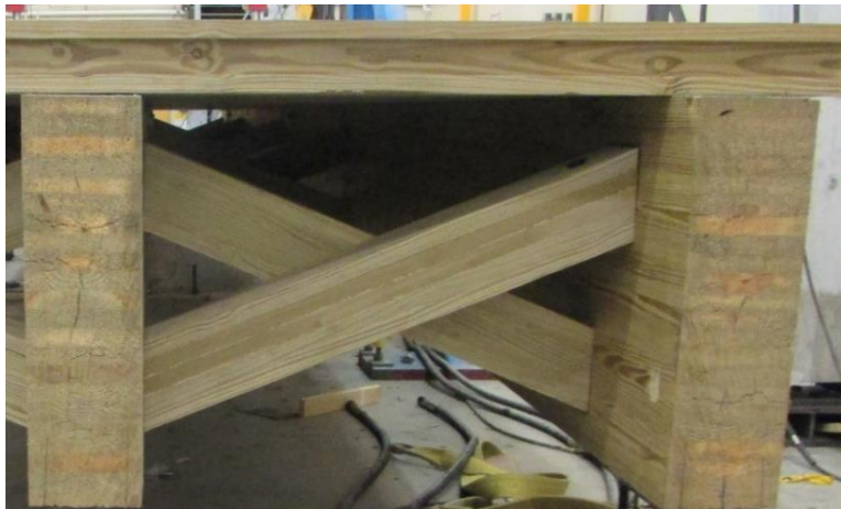
Figure 3.20 Glulam Cross Braces for Girder Timber Bridges
