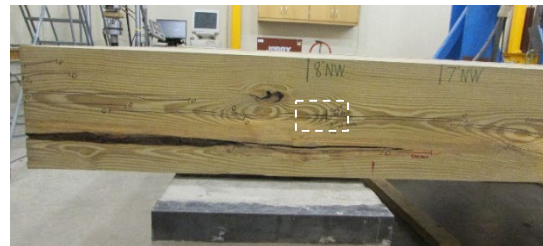
(b) Crack Growth after 550k Cycles – Slab at North Support
