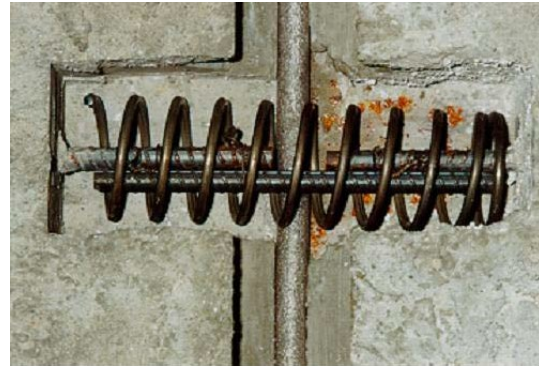
(b) Photogram of Block-out with Tied-in Lap Splice and Spiral Confinement (Badie et al., 1998)
