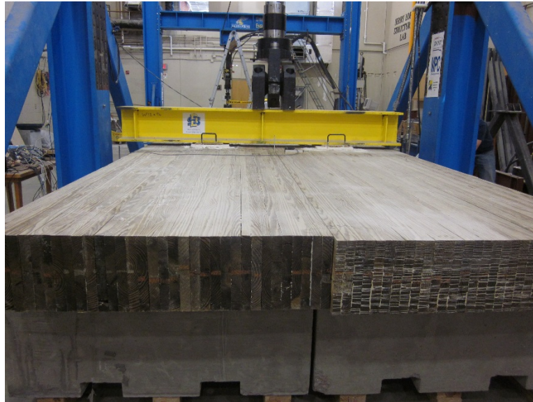
Figure 4.72 Strength Test Setup for Glulam Timber Slab Bridge
