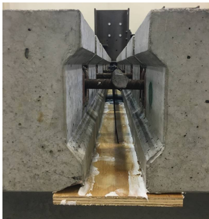
Figure 4.11 Transverse Joint Formwork
