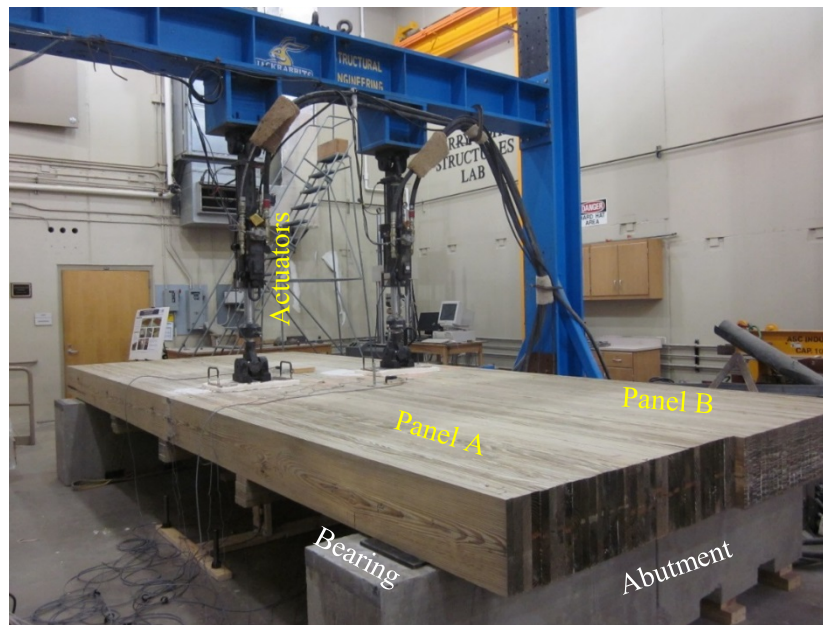
Figure 4.71 Fatigue Test Setup for Glulam Timber Slab Bridge
