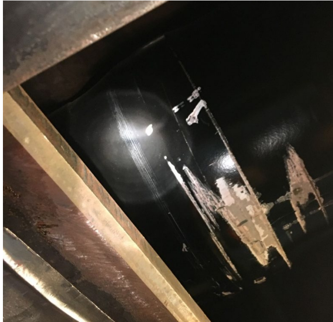
Figure 48. Cracked paint on the right side of the PBC deformation tube, indicating tube crush
