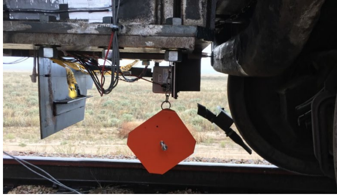
Figure 46. PBC flag detachment indicating the PBC was triggered
