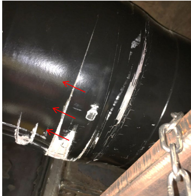
Figure 64. Cracked paint on the left side of the PBC deformation tube indicating tube crush
