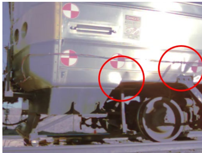
Figure 9. More pronounced dimpling of M1 shell at front-left side sill truck connection after 7.9 mph impact test
