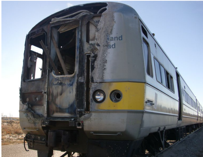
Figure 5. M1 cab car 9324 with some fire damage
