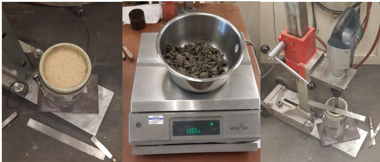
Figure 3.5 Sample Compaction steps (Mebrahtom 2017)
