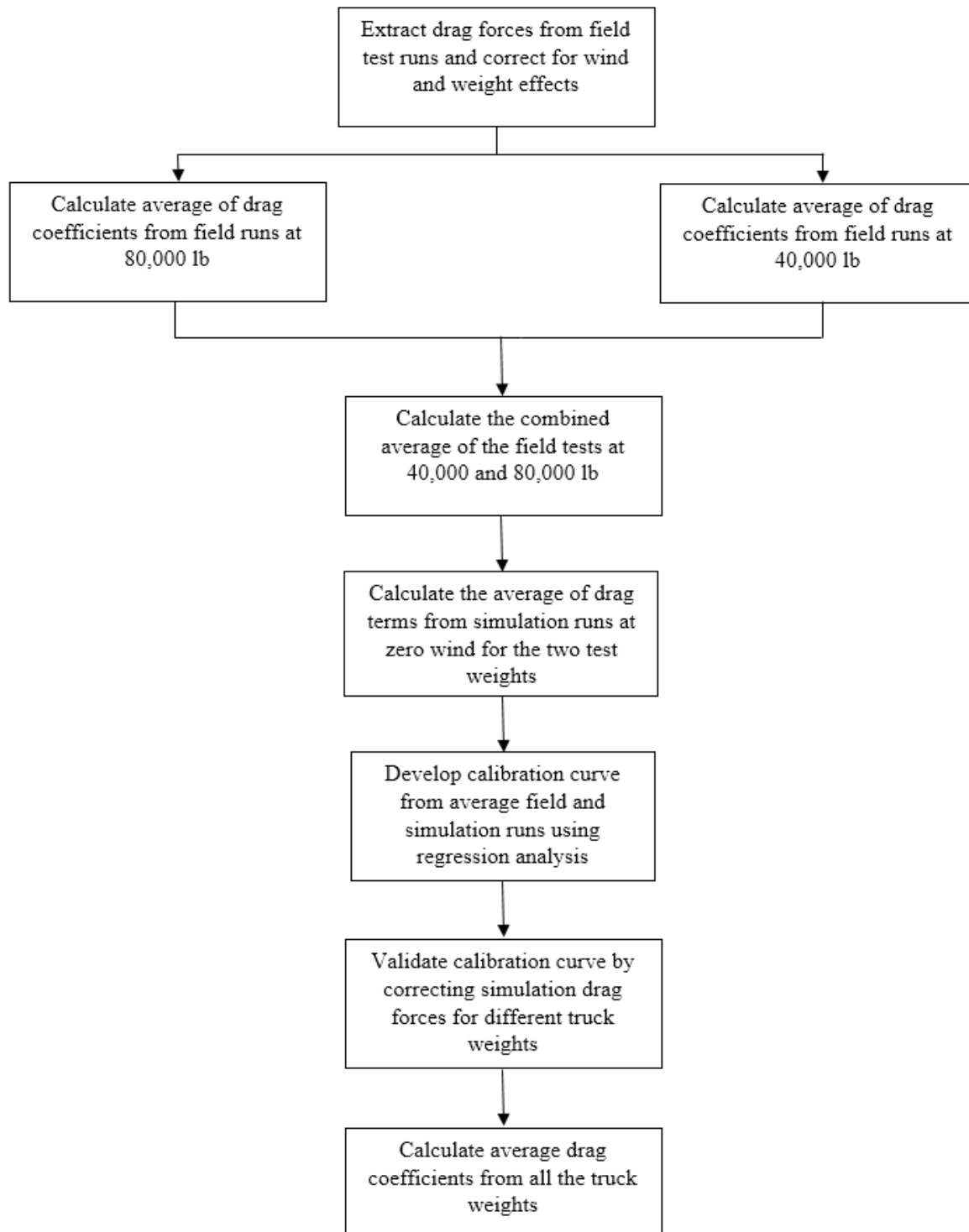
Figure 71. Flowchart for Calibration Curve and Validation.
