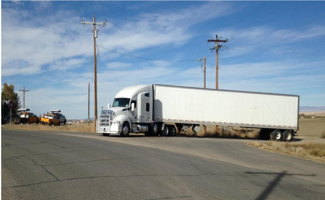
Figure 133. Photo. Truck Turning During Coast-down Testing.
