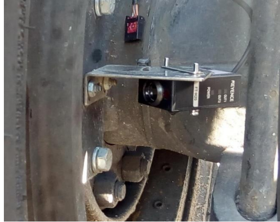
b. Infrared Sensor Installed on Drum.
