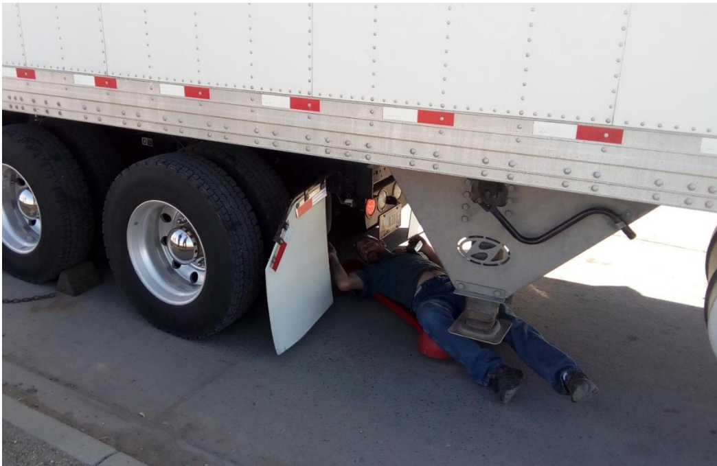
Figure 132. Photo. Technician Adjusting Air Pressure to Brakes.
