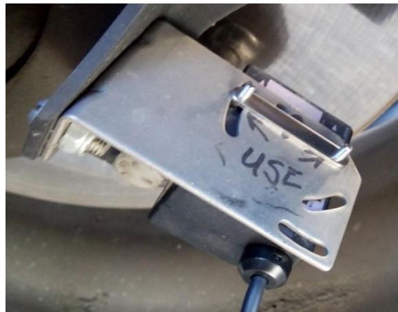
d. Infrared Sensor Installed on Disc Brake
